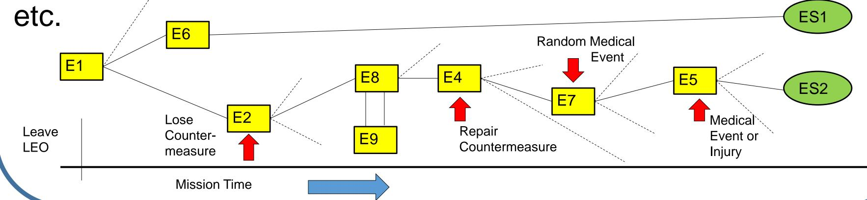
The architecture selected to meet the four significant requirements is a *task queue timeline*, to queue up Event Sequence Diagrams (ESDs), spawn dependent functions, update diagnosis capability, move forward in time, pause to look back in time for group events & hooks to the outside, and purposely send hooks to the outside.
