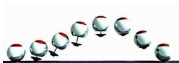
Figure 32: Hopping, spherical robots proposed by (Dubowsky, Iagnemma, & Boston, 2006). Cavehopper exhibits enhanced sensing, control, and efficiency of flat ground driving.
