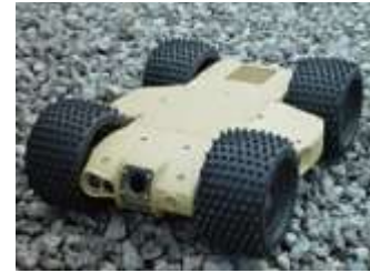
Figure 35: CMU Dragon Runner, a rugged compact robot capable of surviving being thrown off buildings and through windows.
