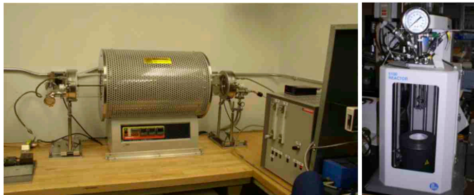
Figure 8. Left: a quartz hydrogen chamber (Carbolite, Ltd.). Right: a pressure chamber (5100 Reactor, Parr Instrument Company).
