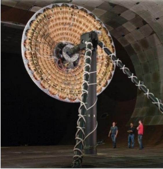
Figure 6: HIAD 6m wind tunnel testing
