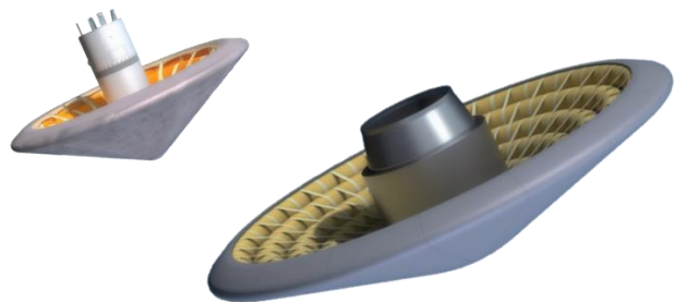
Figure 7: IRVE-3 (3m) to HULA (6m) scale comparison
