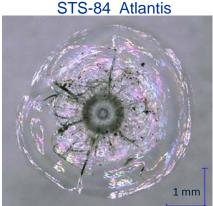
Some windows are not shuttered and can be damaged by MMOD....
