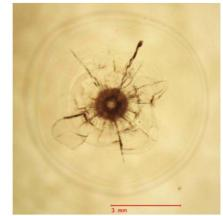
Central pit with radial and circumferential cracks.
