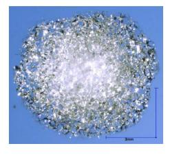
Large pit with gain boundary cracking.
