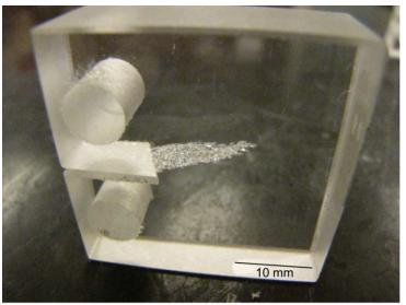
Macro-crack method: direct observation of the crack.
