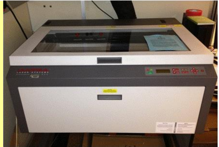
Universal Laser System (Two 60 watt laser heads and a work area of 32"x18")
