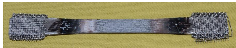
PVD GdYSi coated on Hyper Them 12C-461-002_#17 1316°C, 10ksi, 1000 h fatigue (3 Hz, R=0.05)
