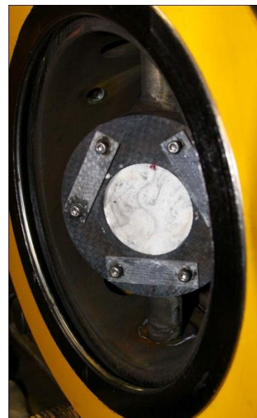
2" diameter ND3 EBC/SiC/SiC specimen after testing in the high pressure burner rig At 2600°F
