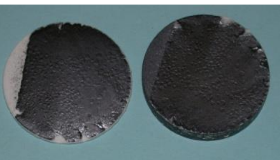
Si bond coat after 1350°C, 50 hr furnace test in air; 1" dia plasma sprayed EBC button specimen
