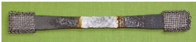
APS Bond Coat series on CVI-MI SiC/SiC EBC at 1400°C, 10 ksi, 400 hr
