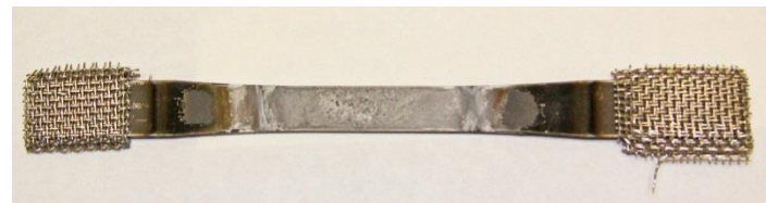
1316°C, 15ksi, 1169 h fatigue (3 Hz, R=0.05) on GE Prepreg SiC/SiC
