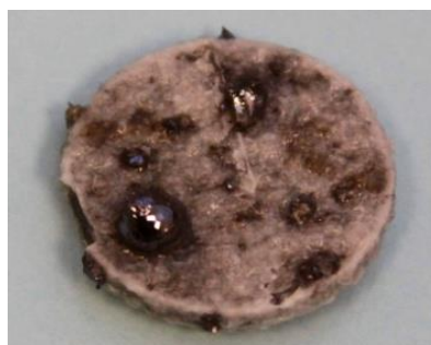
Hot pressed BSAS+Si button specimen after 1350°C, 50 hr furnace test in air
