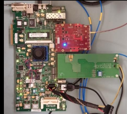
Merged RF & optical waveform control on COTS development board
