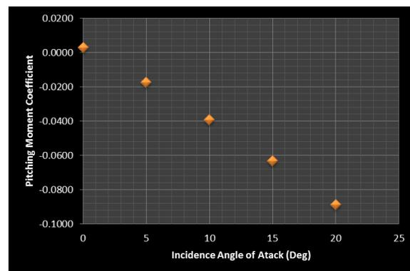
**Figure 10: Static stability condition is satisfied for MIRCA**
