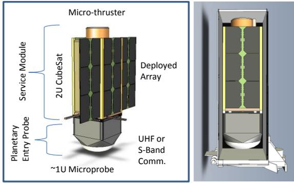
**Figure 1: CAPE in its deployed configuration, and stowed inside deployment system**
