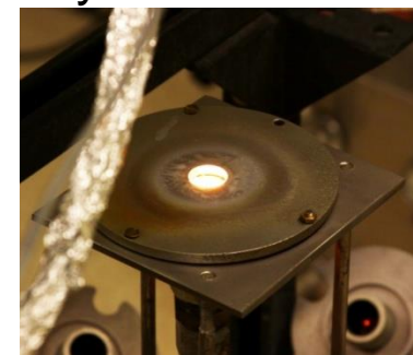
The EBC-CMC specimen under testing
