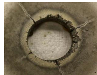
Tested EBC-CMC specimen tested for 500 hr durability
