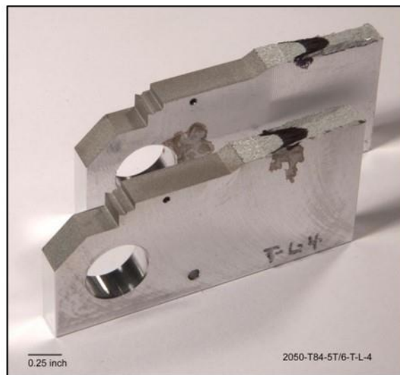
Figure E5. Fracture toughness data, J-curve, and image showing fracture path for 2050-T84, T-L orientation, 5t/6, specimen 4, tested at 75°F.
