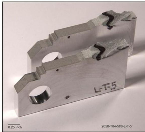
Figure E2 Fracture toughness data, J-curve, and image showing fracture path for 2050-T84, L-T orientation, 5t/6, specimen 5, tested at 75°F.
