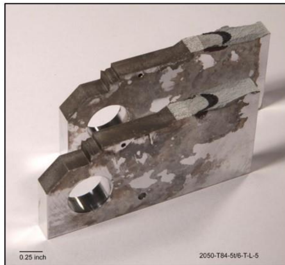
Figure E12. Fracture toughness data, J-curve, and image showing fracture path for 2050-T84, T-L orientation, 5t/6, specimen 5, tested at -320°F.
