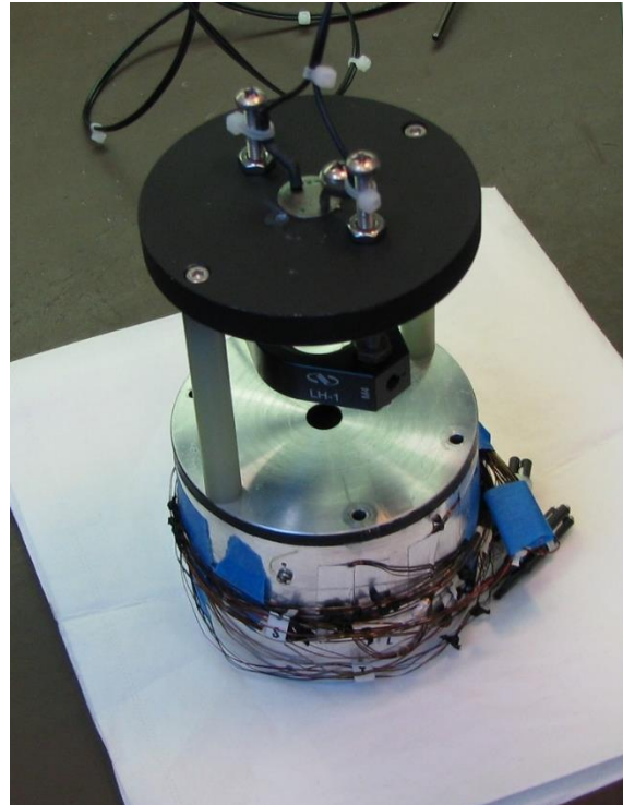
Light source and lens launching radiation into the cold cell
