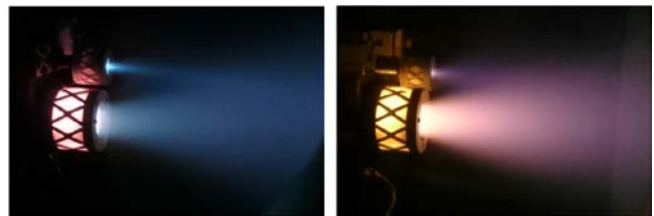
Figure 10. BIT-3 RF Ion Thruster during ground testing: Xenon (left), Iodine (right) [20]
