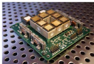
Figure 13. S-iEPS 8 thruster array mounted on PPU [21]
