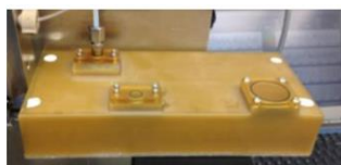
1.5kg-Capacity, Thermoplastic Solid Iodine Storage Tank; 22psi Proof Pressure
