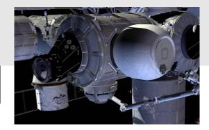
Outfitting ISS for the arrival of commercial crew visiting vehicles (VV) includes reconfiguring ISS to accommodate two VV docking ports and two VV berthing ports
