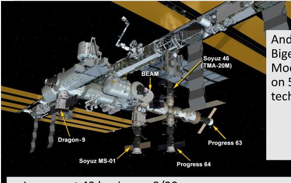
And, the first inflatable module, Bigelow Expandable Activity Module, or BEAM, was inflated on 5/28, starting a 2-year technology demonstration
