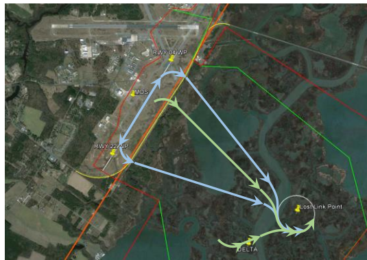
Figure 8. Illustration of CS-A trajectories from several potential activation locations to the lost link point.
