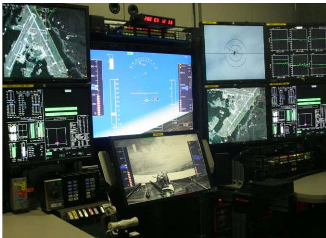
Figure 6. Photo of the remotely piloted airplane cockpit located in the AirSTAR mobile operations station.
