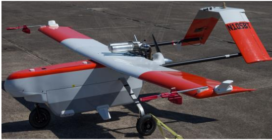
Figure 1. Photo of remotely piloted airplane used for test of the AirSTAR beyond visual range system.
