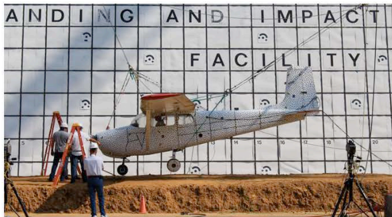
Figure 1. Pre-test photograph of C-172 crash Test 2 airplane at impact attitude.
