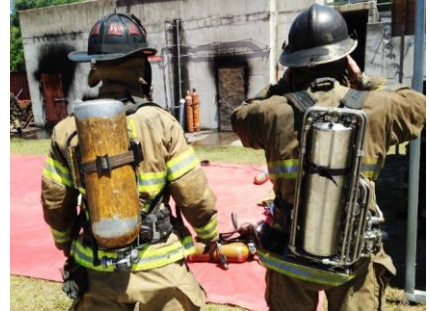
Comparing the advanced cryogenic breathing apparatus to traditional self-contained breathing apparatus in firefighting applications
