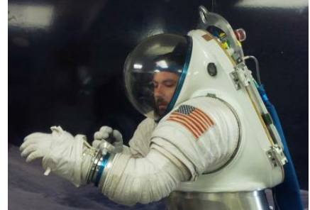
Form, Fit, and Function Testing of EVA Swab With Mark III Suited Subject
