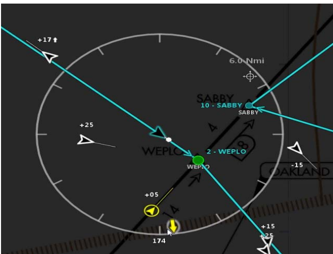
Figure 3. Lateral Vector Planning tool during a Preventive DAA alert. Solid yellow arrow indicates the specific heading selected (174°) will lead to a Corrective DAA alert if flown.
