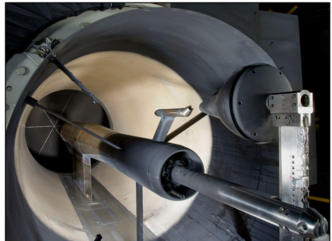
Figure 3-8: Single AM nozzle with LAV body mounted downstream at NASA Glenn Research Center[19].
