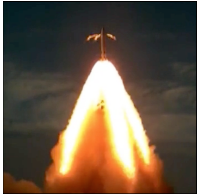
Figure 3-7: Abort and Attitude Control Motors firing during a pad abort test of the Orion[18].
