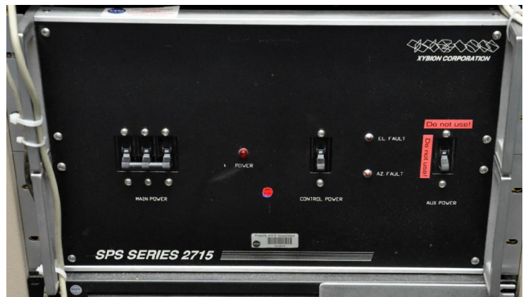
Figure 3-8: Controller for the mount, located in the equipment rack behind the operator
