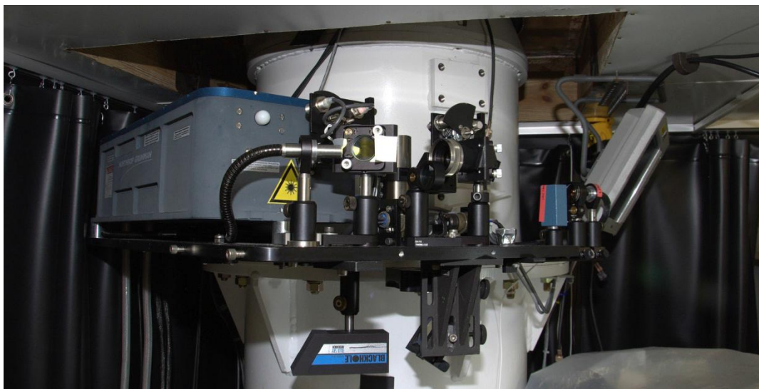
Figure 3-11: LRO Laser and LRO Optical Table mounted on the Telescope Pier above the SLR Optical Bench
