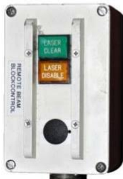
Figure 8-5: Beam Block Control Box
