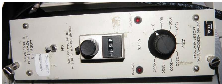
Figure 3-23: Bertran High Voltage Power Supply
