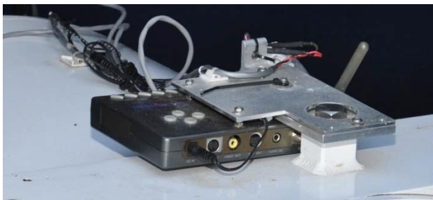
Figure 8-3: Wireless transmitter for the Mount Camera
