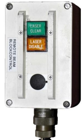
Figure 15: Remote Beam Block Control box
