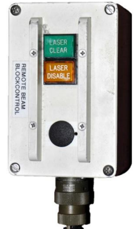
Figure 15: Remote Beam Block Control box
