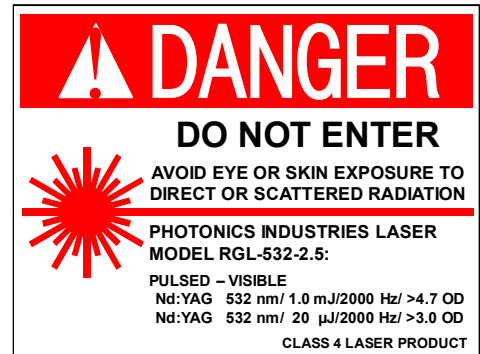
Figure 3-6: PI Laser Warning Sign
