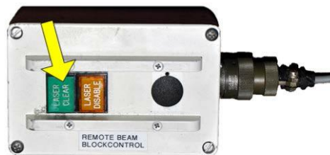
Figure 10: Remote Beam Block Control Box
