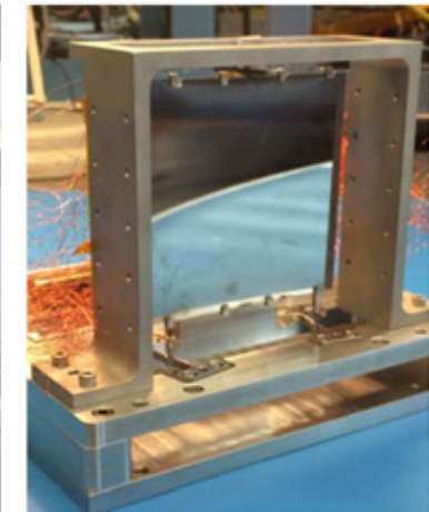
Single shell mounting concept with a mounted adjustable mirror
