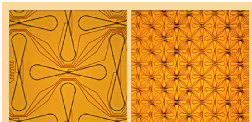
Fig. 6. Left: Broadband 200-300-GHz antenna designed from a unit “bowtie” sub-antenna. The bowtie is a slot design in a base Nb ground plane, back-illuminated through the Si wafer. The sub-antennas connect to a feed network of microstrip lines. Right: A larger-scale view of the broadband antenna, showing the combination of sub-antennas. The design detects vertical polarization in horizontal bowties, which are interleaved with the two feed networks.
