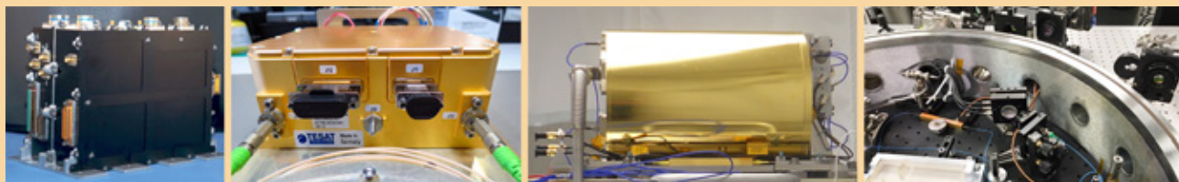
Fig. 1. The LRI design requirements and designs came from US and German investments in GW technology as well as geodesy. LRI hardware shown (left to right): Laser Ranging Processor (LRP), Laser, Optical Cavity, and Optical Bench Assembly (OBA).
