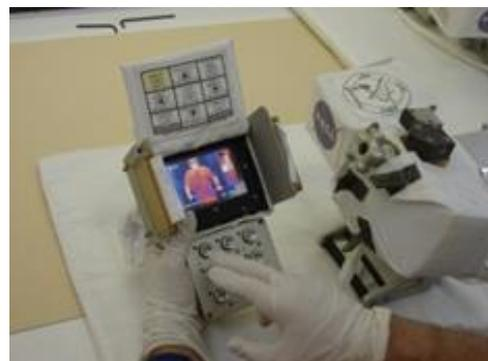
Fig. 4 Infrared inspection system designed for on-orbit inspections.
