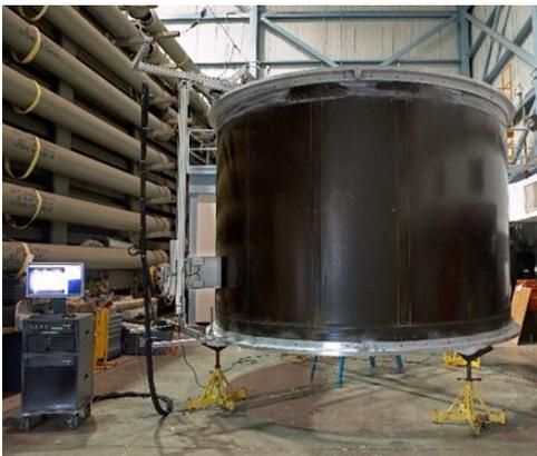
Fig. 2 System configured for large area inspection of a composite test article.
