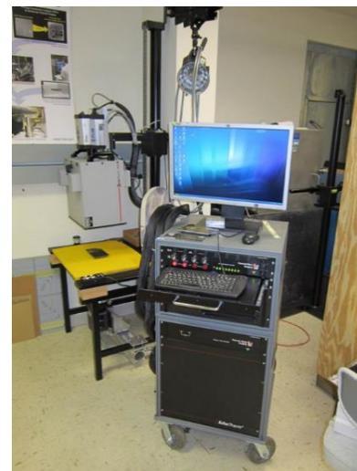
Fig. 1 Photograph of the flash thermograph system.
