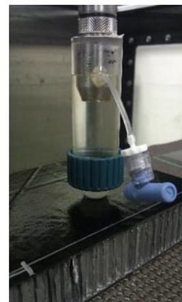
Fig. 6 A photograph of a single-element transducer with a captive water column used for large area, high speed ultrasound.
