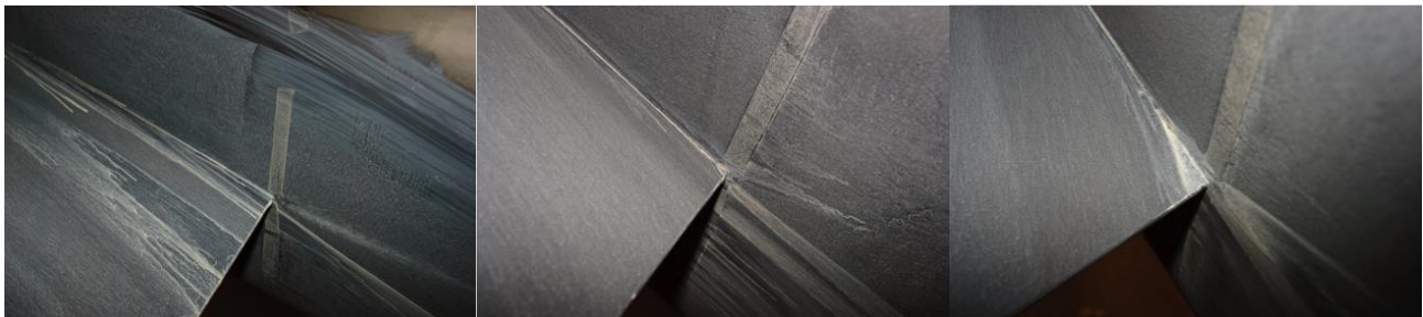
Figure 1-6: Oil flow patterns from the 0015-based wing, angles of attack = 0, 5, and 10 from left to right.
