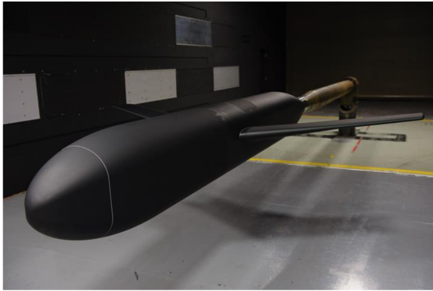
Figure 1-4: Photograph of 6%-scale JF model in the NASA Langley 14x22 wind tunnel.
