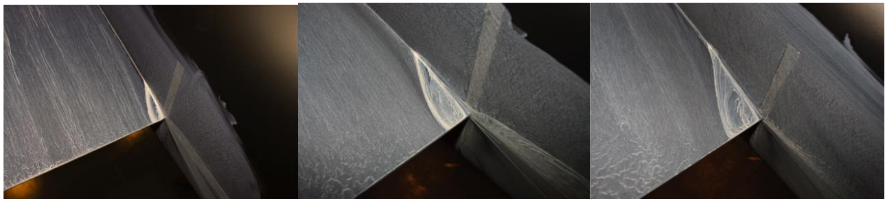
Figure 1-5: Oil flow patterns from the F6 wing (6%-scale model), angles of attack = 0, 5, and 10 from left to right.
