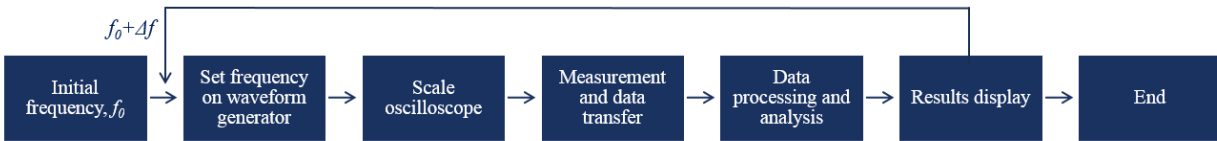
Figure 2. Automated algorithm for data collection and analysis of guided waves for in-process cure monitoring.
