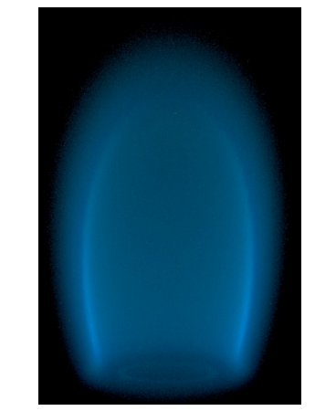
Fig. 1: Example of blue chemiluminescent emission from a nitrogen-diluted methane diffusion flame
