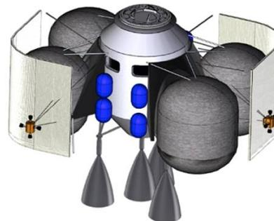
Mars Ascent Vehicle (MAV) 2-stage, pump-fed engine concept (Incorporates ISRU generated LOX)
