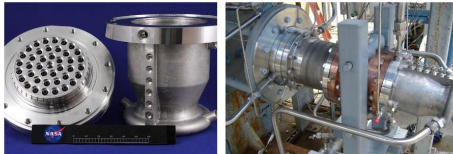
MSFC Additively Manufactured 4 Kibf LOX/LCH4 Engine
