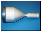
440 N LMP-103S thruster during manufacturing at Plasma Processes Inc.
