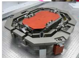
Fold Mirror 3 Tip/Tilt Gimbal Assembly
