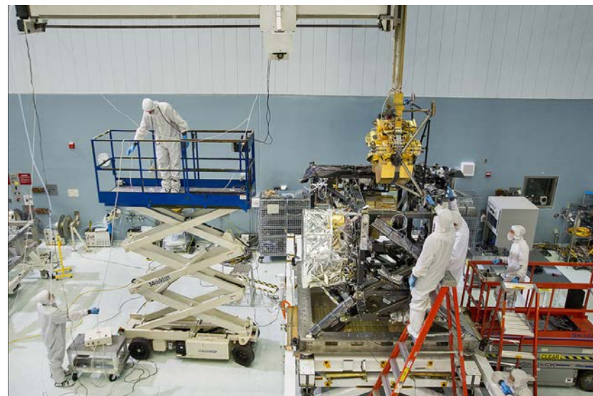
Integration of science instrument optical assemblies
