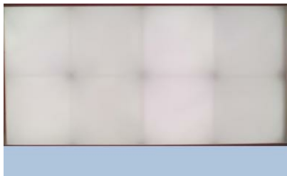
True Color image of the light panel system with a large diffuser sheet mounted in front.
