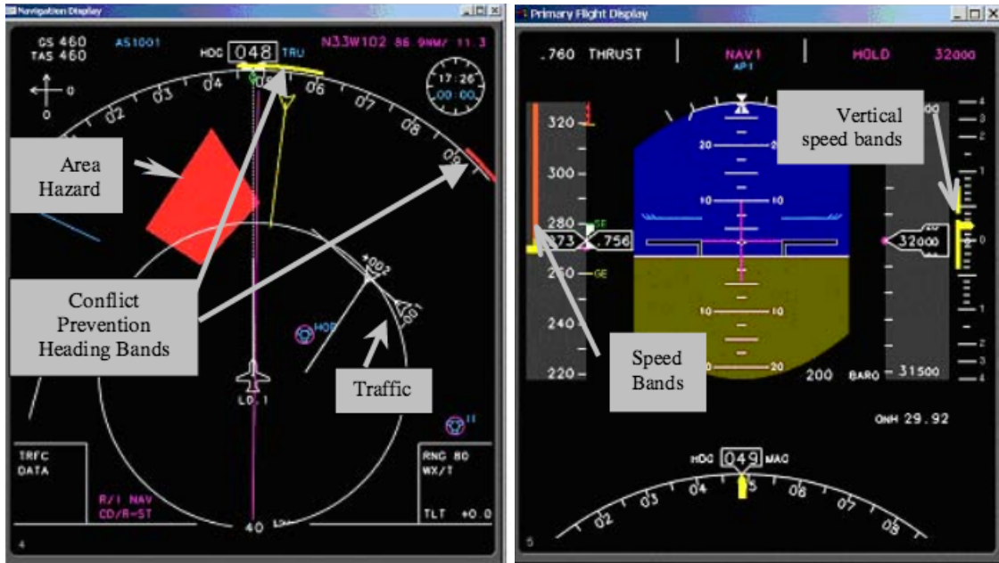
Figure 39. Illustration of NASA Langley Research Center's conflict prevention heading (right) and vertical speed (left) bands. Conflict prevention bands were generated by the prototype autonomous operations planner. Images reprinted from Mondoloni, Palmer & Wing (2002), Development of a Prototype Airborne Conflict Detection and Resolution Simulation Capability.
