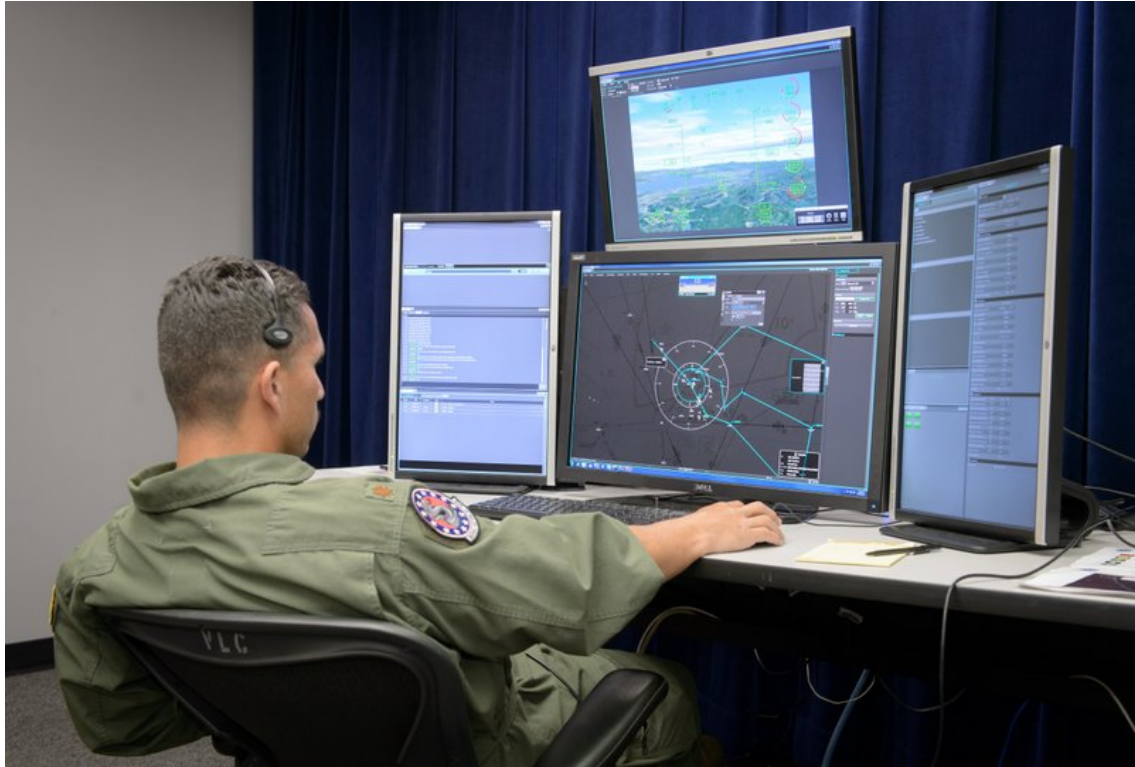
Figure 45. Experimental ground control station. TSD, bottom-center; health and status panels, bottom-left and right; out-the-window view, top center.
