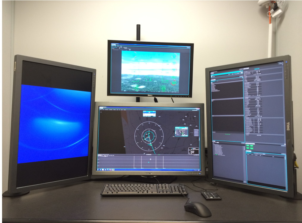
Figure 15. UAS GCS. CSD (not displayed), bottom left; TSD, bottom center; out-the-window view, top center; health and status panel, bottom right.
