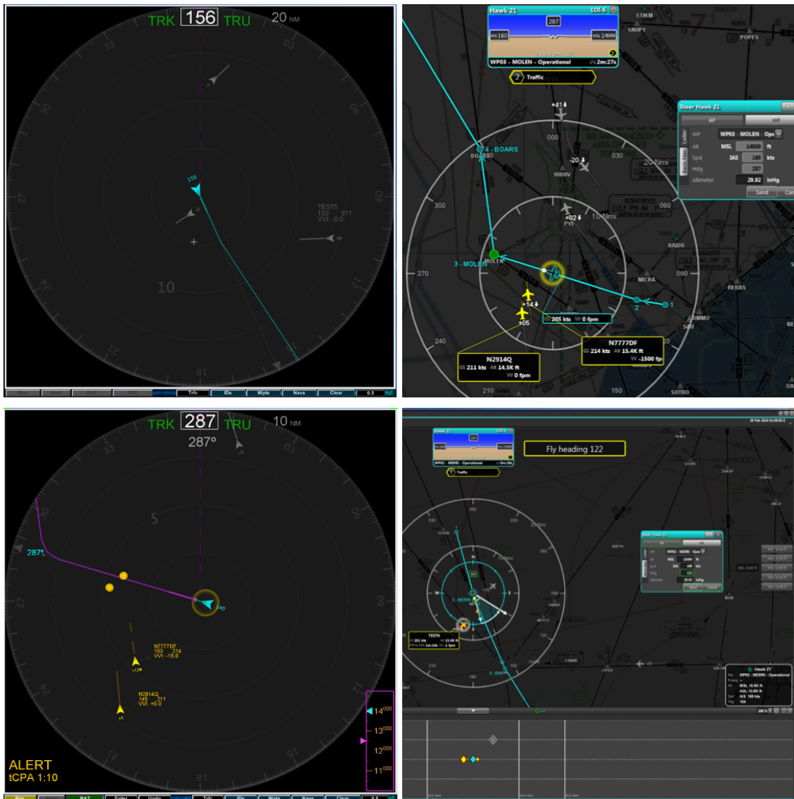
Figure 10. The four DAA displays that were evaluated in Experiment 1: Standalone Basic (top left), Integrated Basic (top right), Standalone Advanced (bottom left), and Integrated Advanced (bottom right).
