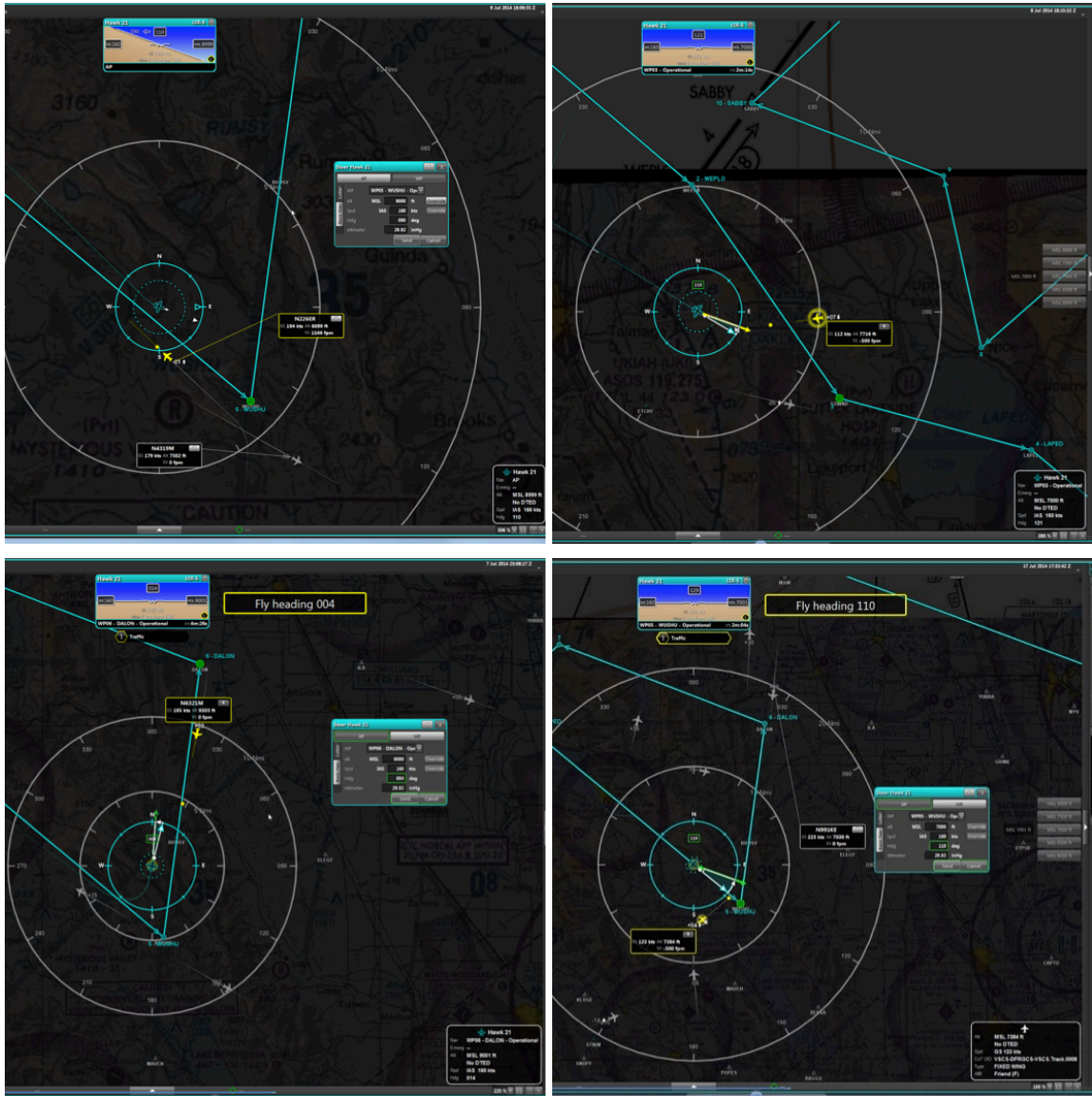
Figure 26. The four DAA displays that were evaluated in Experiment 2: Info Only (top left), Info + Vector (top right), Info + AR (bottom left), and Info + Vector + AR (bottom right).
