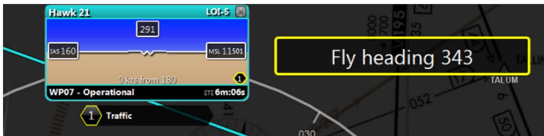
Figure 28. The auto-resolution text box providing directive guidance, here, “Fly heading 343.”
