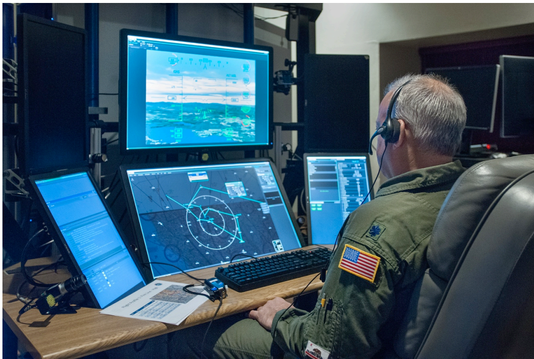
Figure 29. UAS GCS set up for Experiment 2; TSD, bottom center; out-the-window view, top center; health and status panel, bottom right and bottom left.
