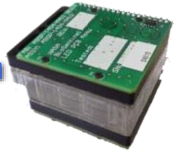
Development Fluidic Card with Optical Detection System
