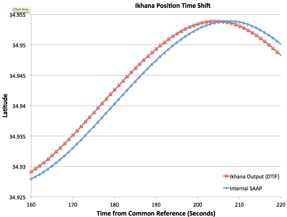
Figure 21. Comparison of the Ikhana self-reported location vs. the post processing of the internal SAAP data from the Ikhana. The Ikhana output is shifted by approximately 3 seconds early (to the left).
