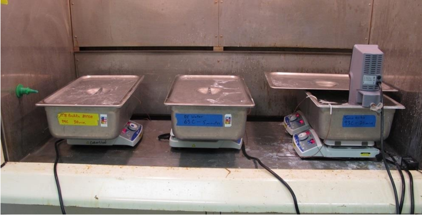
Figure 2 – Test Panels Soaking in Citric Acid Passivation
