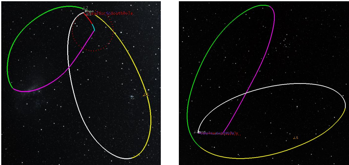
Figure 13. Direct TLI CCAFS South pole impact case shown through sample-return to Earth. Solution shown in the Earth inertial frames (normal to the lunar orbit plane on the left, and edge-on the lunar orbit plane on the right). Highest apogee altitude is 2.35 million km.
