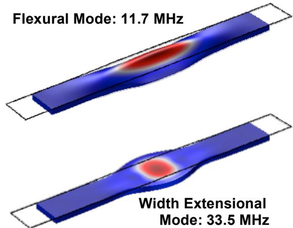
*Simulated mode shapes for the proposed dual-mode architecture. The top mode is a flexural mode, which resonates at 11.7 MHz. The bottom mode is a width extensional mode which resonates at 33.5 MHz.*
