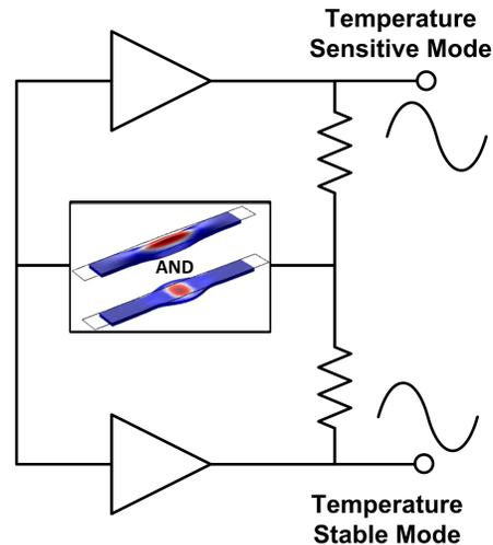
*A schematic of the proposed dual mode architecture. One mechanical resonator outputs two timing signals, one that is temperature stable for use as a reference and one temperature sensitive signal for use as a sensor.*
