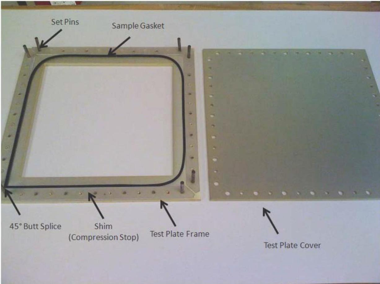
**Figure 4 - Example of CHO-TP09 Test Plate Set**
