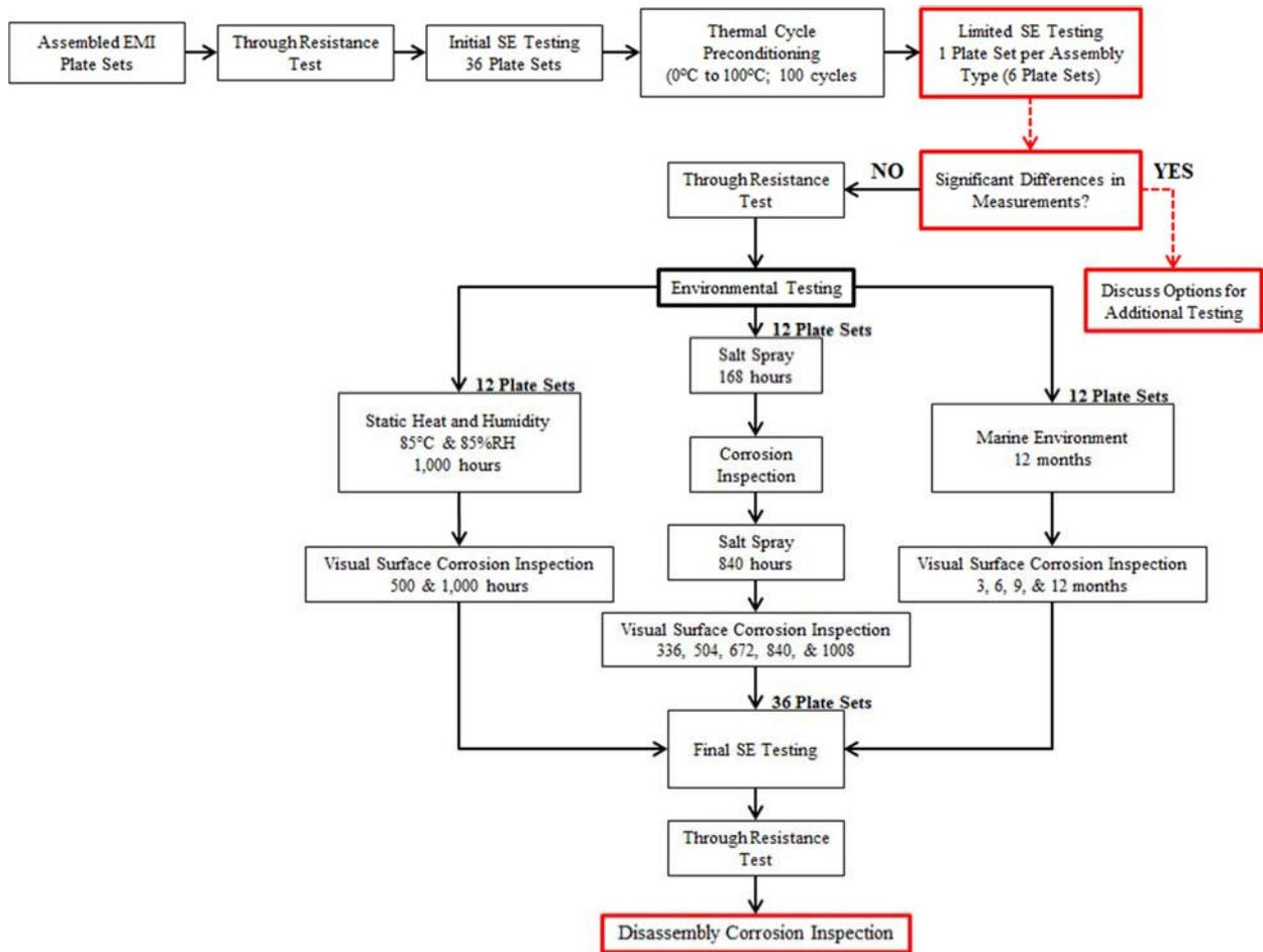
**Figure 5 – Plate Set Testing Project Flow**
