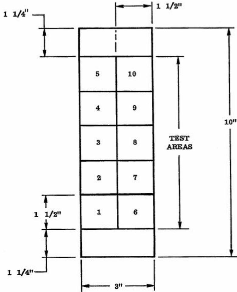
**Figure 13 - Contact Electrical Resistance Test Pattern**
