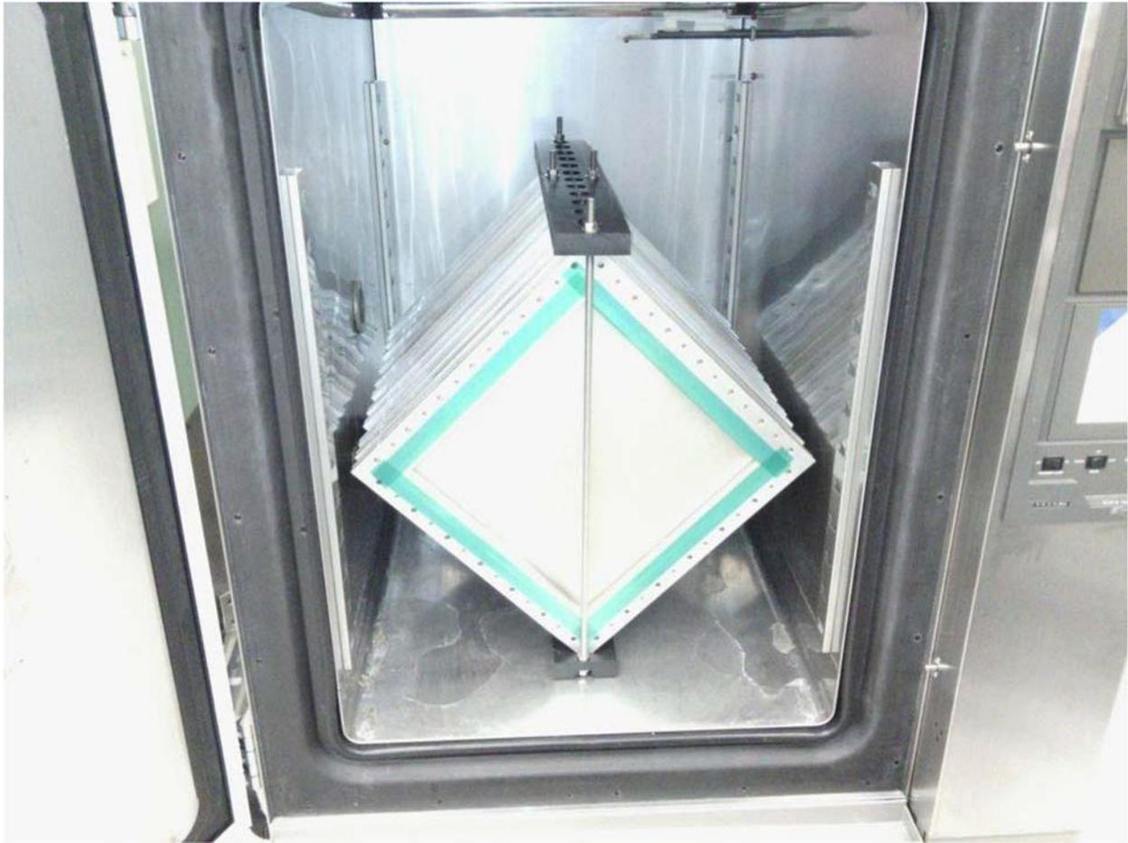
**Figure 9 – Static Heat and Humidity Test Setup**
