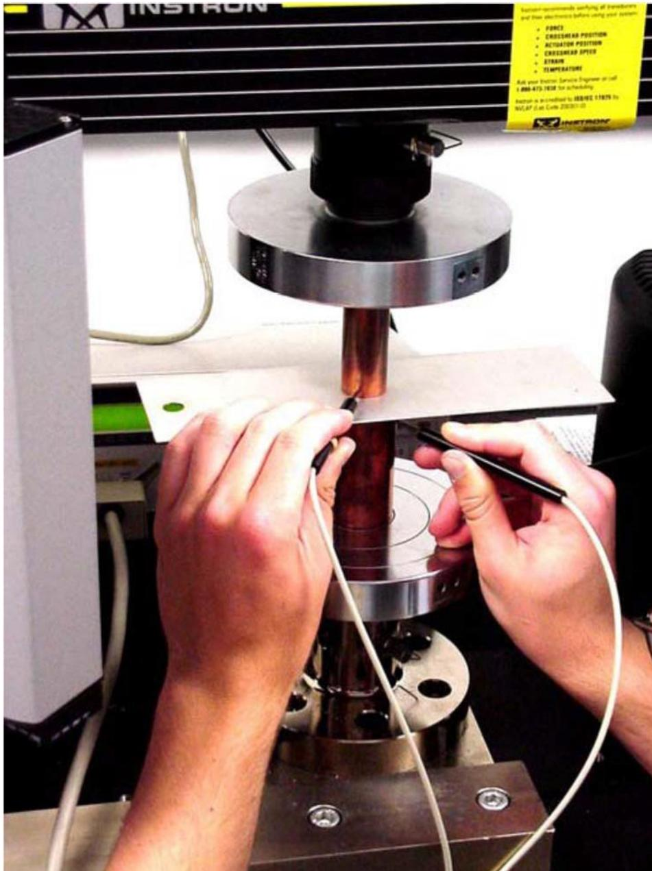
**Figure 12 - Contact Electrical Resistance Testing**
