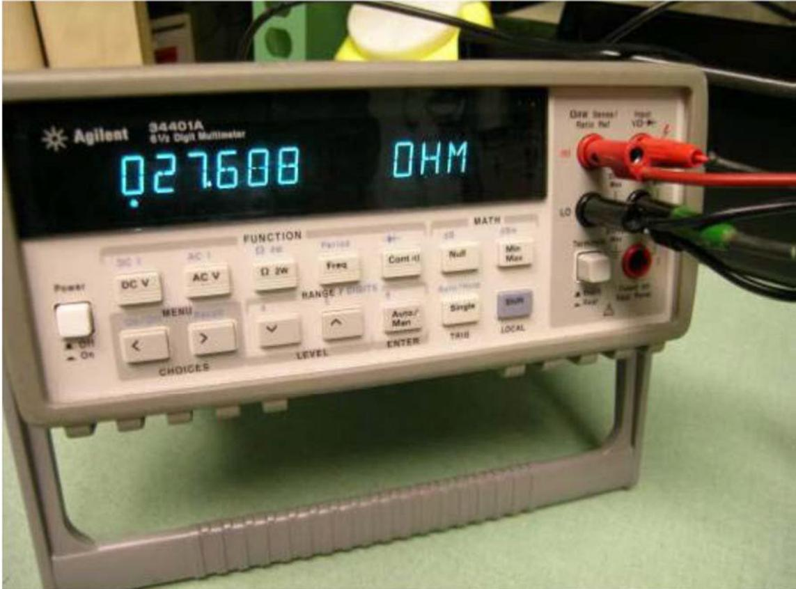
**Figure 14 – Surface Resistance Test Set-Up**
