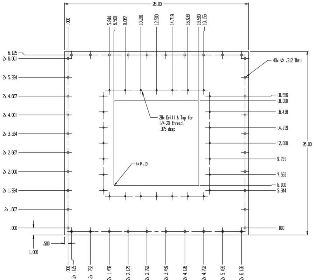
**Figure 3 - Main Adapter Plate for Mounting Test Plate Sets to Wall of Shielded Enclosure**
