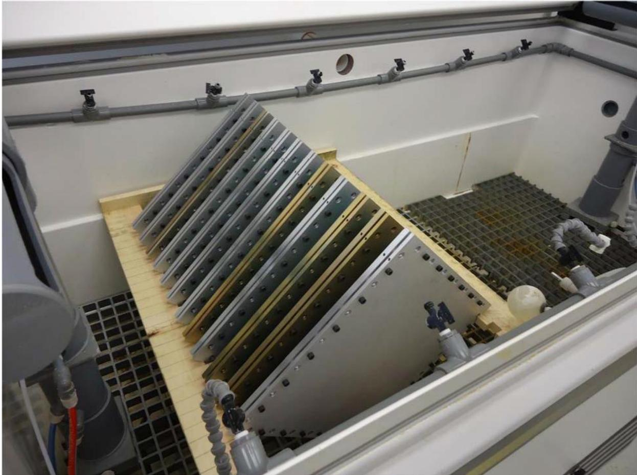
**Figure 8 – ASTM B 117 Salt Spray Setup**
