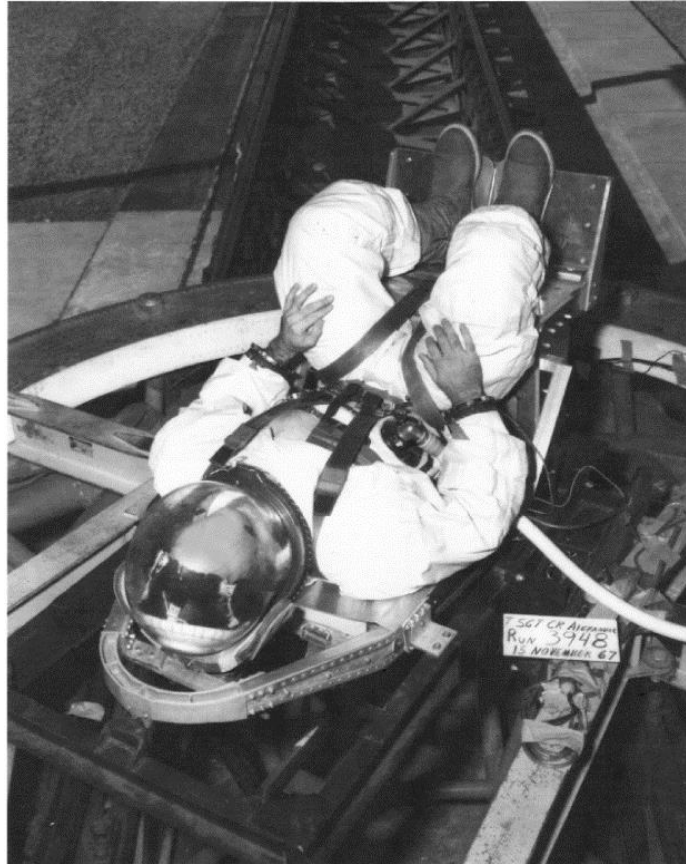
Figure 3.1-9. A Volunteer Being Tested in a Developmental Pressure Suit (credit: USAF)
