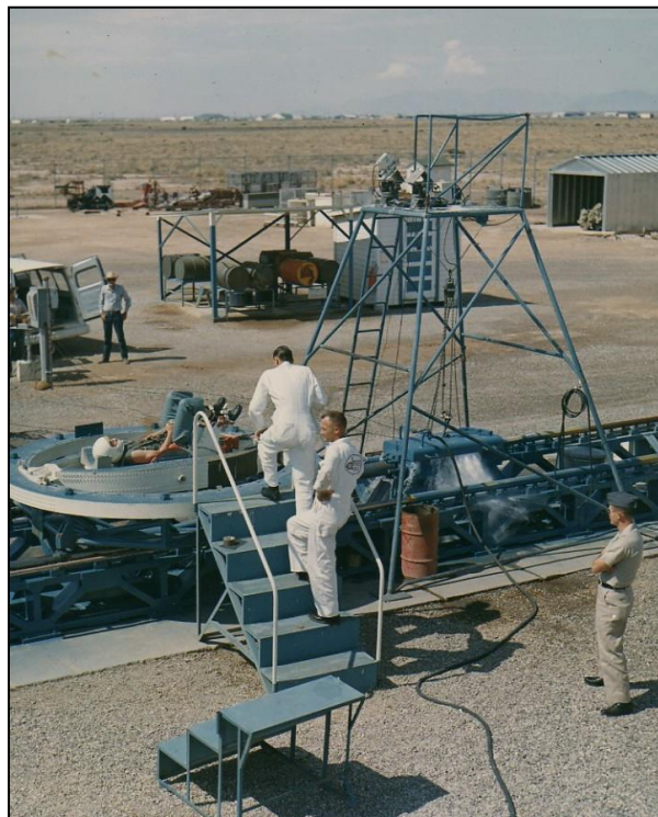
Figure 3.1-6. Photograph of Horizontal Deceleration Test Facility and Subject Restrained within the Multi-directional Test Apparatus
