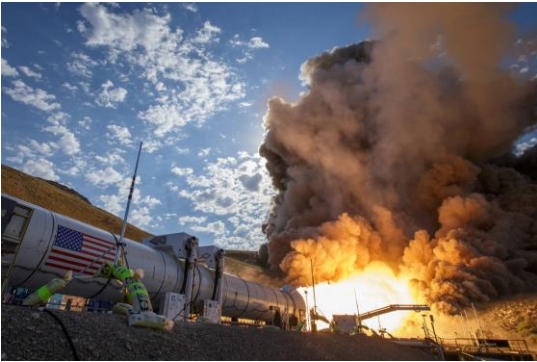
Figure 4: Qualification Motor-2 test of the SLS solid rocket boosters.
