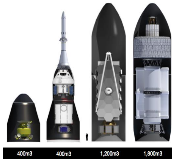
Figure 8. Fairing options for evolved configurations of Space Launch System.
