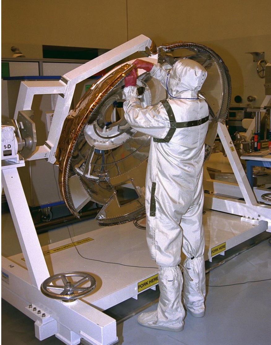
Figure 6.4 A worker repairs the multi-layer insulation on the Huygens probe after an abnormally high pressure purge ripped the delicate material.
