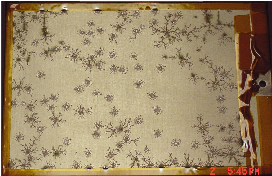
Figure 6.3 Breakdown of anodized aluminum in plasma environment
