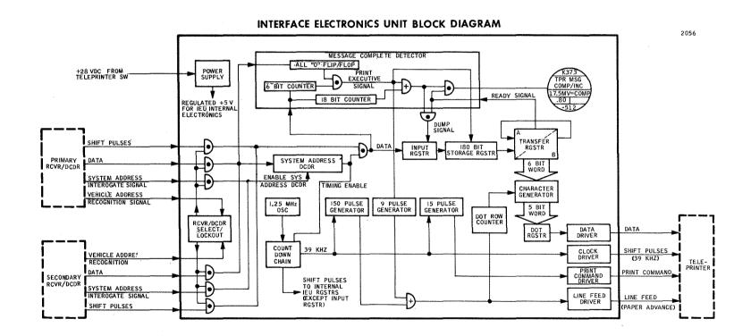
Figure 2.2.4-3 Interface Electronics Unit Operation
