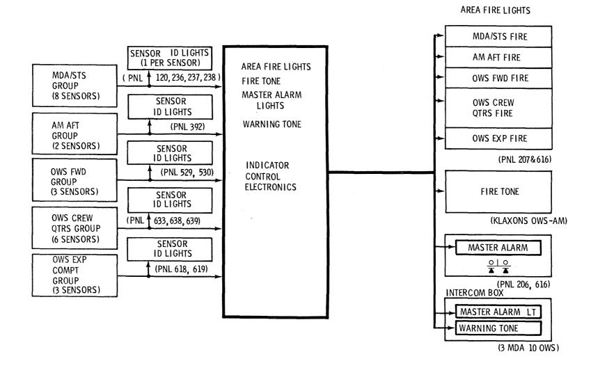
Figure 2.8.3-6 Fire Detection Subsystem
