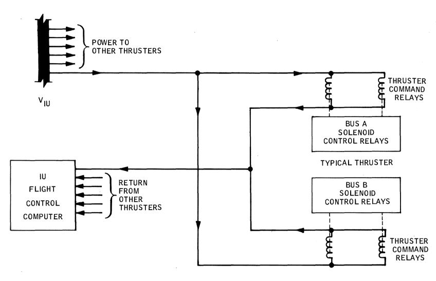
Figure 2.3.3-7 IU Command/Thruster Interface
