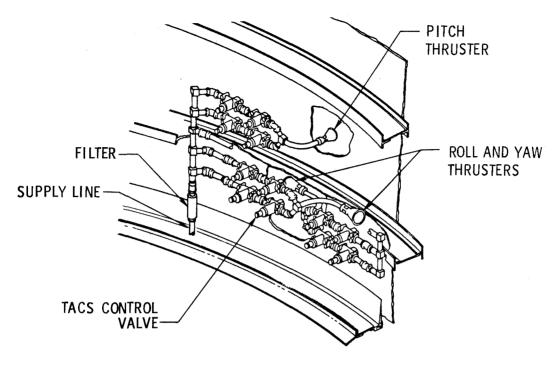
Figure 2.3.4-1 Control Valves Internal View
