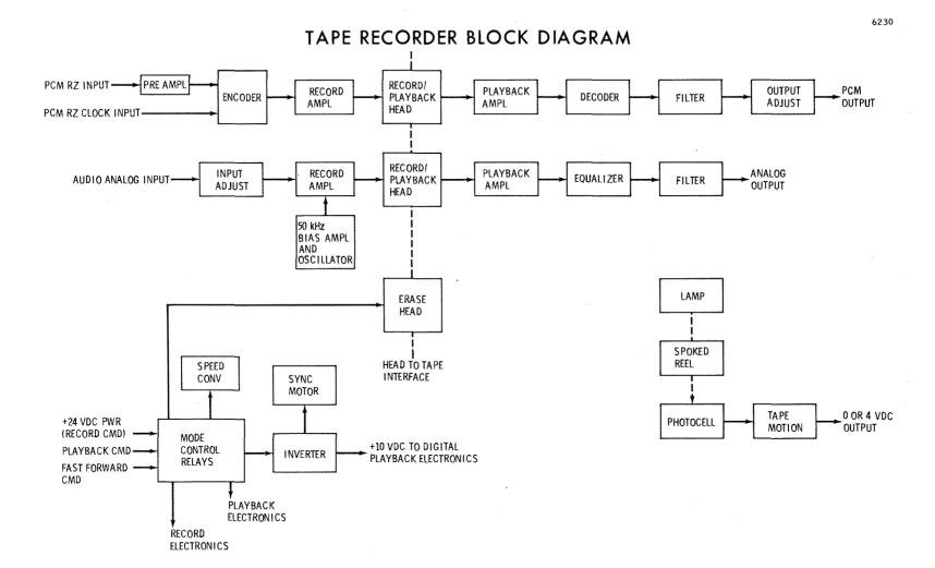
Figure 2.6.4-18 Tape Recorder Block Diagram
