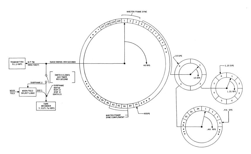
Figure 2.6.3-8 PCM Format (Sample Rates)
