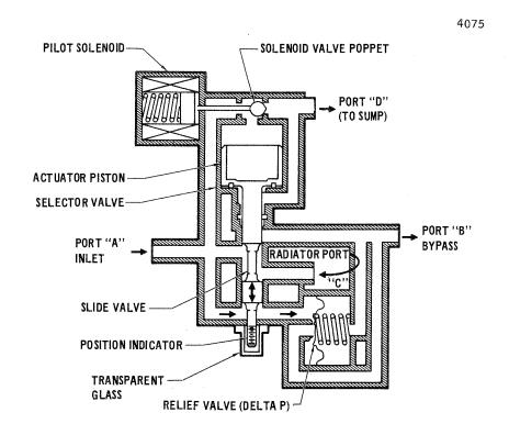
Figure 2.4.4-41 Radiator Bypass and Relief Valve
