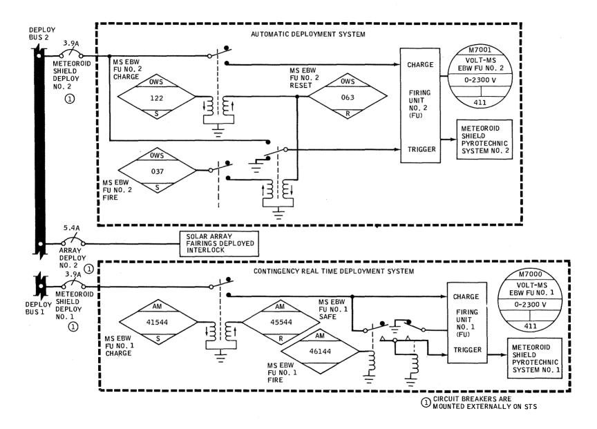
Figure 2.0.10-36 Meteoroid Shield Deployment System
