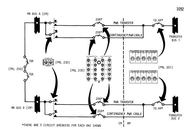
Figure 2.1.3-17 AM/CSM Distribution Interface
