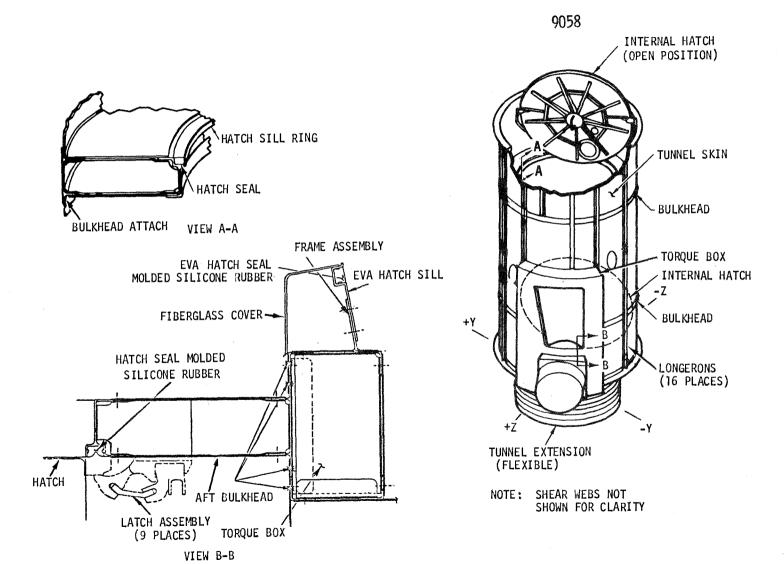
Figure 2.0.8-8 Tunnel Assembly
