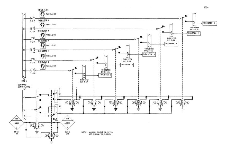
Figure 2.3.3-6 Bus 1 On/Off Command -- Schematic
