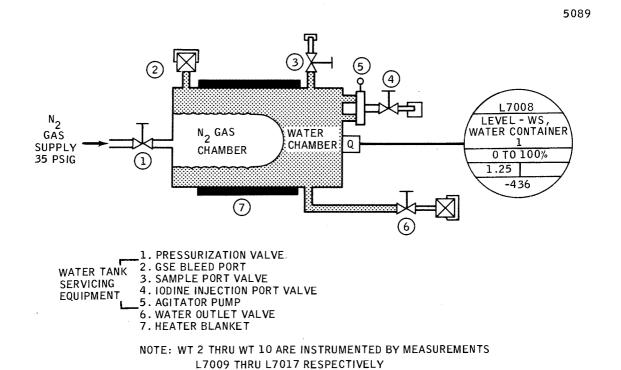
Figure 2.5.12-4 Typical Water Tank -- Schematic
