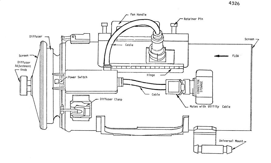
Figure 2.4.4-57 Portable Fan Assembly
