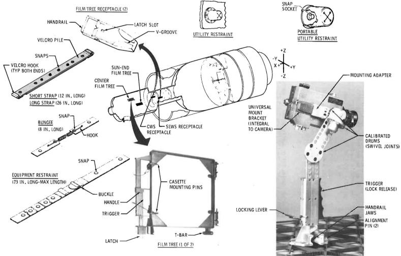
Figure 2.5.3-5 Equipment Restraints - Internal
