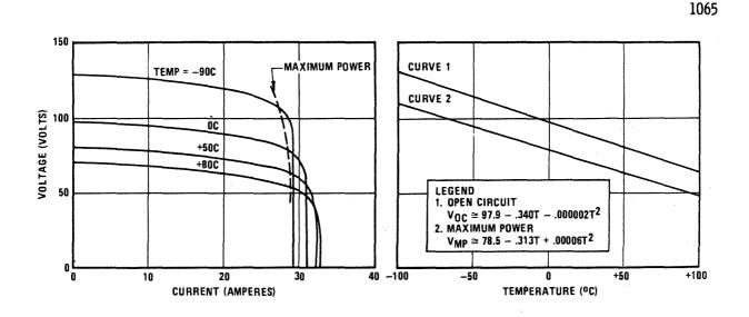
TYPICAL FOR SOLAR ARRAY GROUP (30 SOLAR CELL MODULES)
