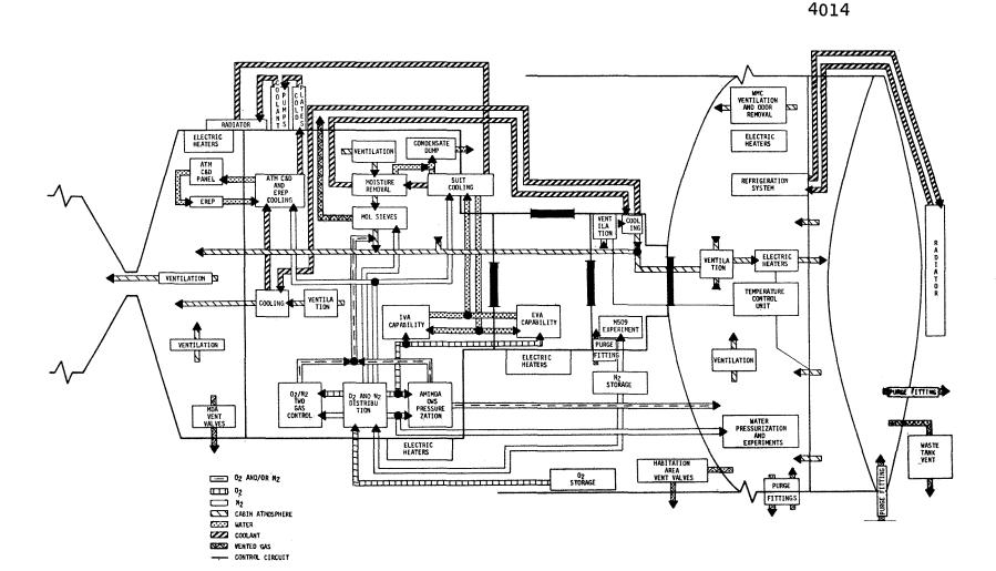
Figure 2.4.1-2 ECS Flow Diagram
