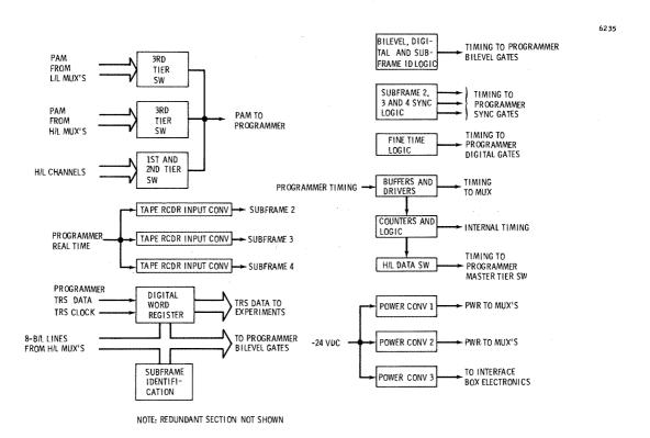
Figure 2.6.4-13 Interface Box Block Diagram
