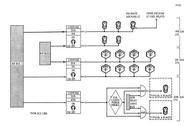
Figure 2.5.4-6 EVA Lighting -- Functional Diagram
