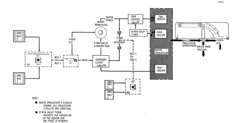
Figure 2.5.11-12 Typical Waste Processor -- Functional Diagram
