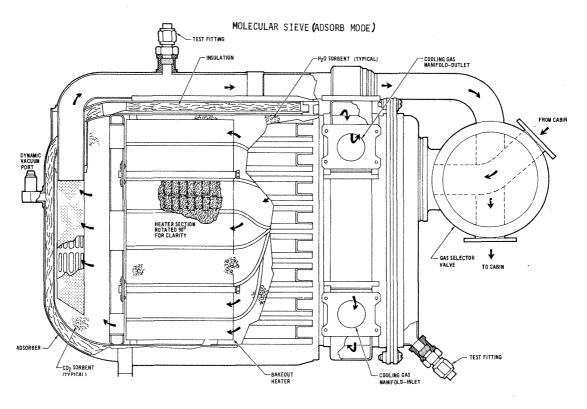
Figure 2.4.4-69 Molecular Sieve Sorbent Canister
