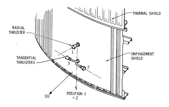
Figure 2.3.3-1 Thruster Attitude Control System Thruster Module
