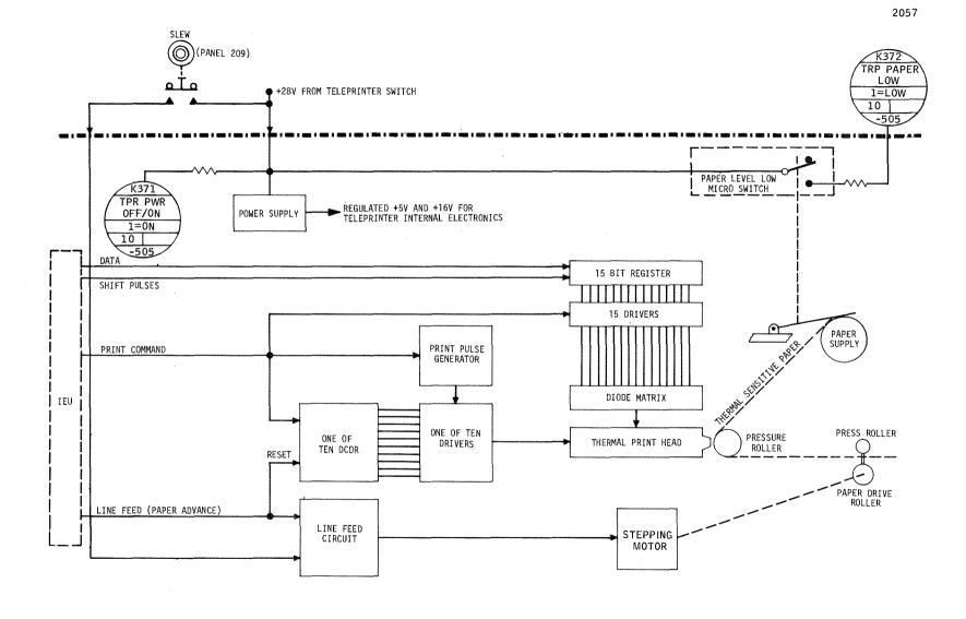
Figure 2.2.4-4 Teleprinter Operation
