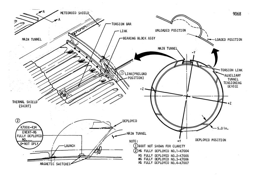
Figure 2.0.10-34 Meteoroid Shield Deployment Mechanism
