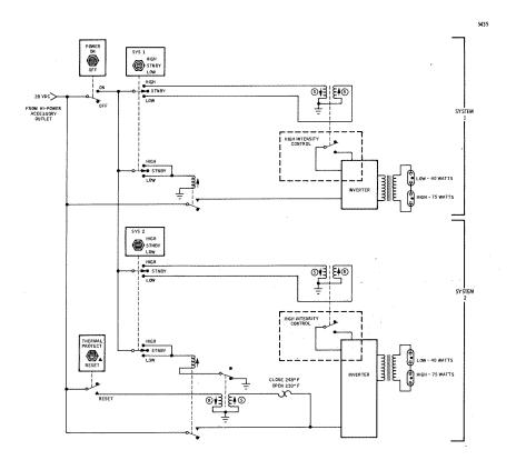
Figure 2.5.4-21 High-Intensity Light -- Schematic
