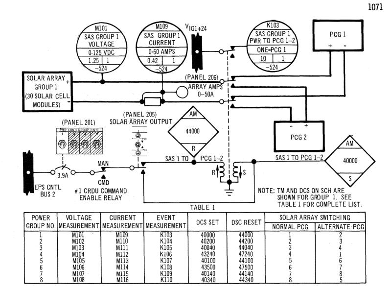
Figure 2.1.3-5 Typical Solar Array Group/PCG Interface
