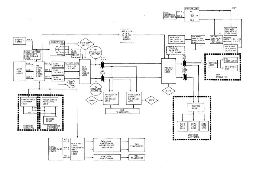
Figure 2.6.3-2 Power Subsystems
