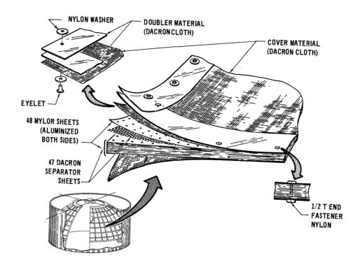
Figure 2.4.4-32 High-Performance Insulation
