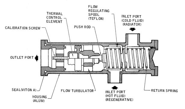
Figure 2.4.4-44 Temperature Control Valve -- 40°F
