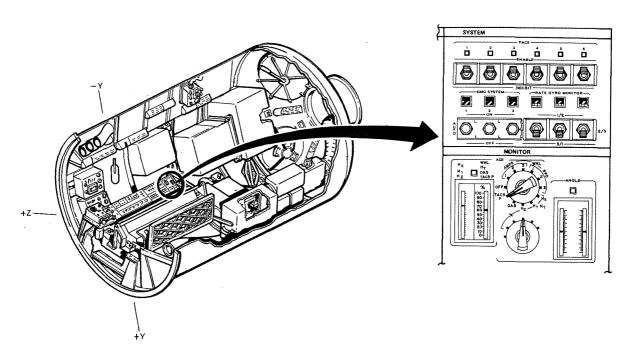
Figure 2.3.3-11 Manual Inhibit Control Panel
