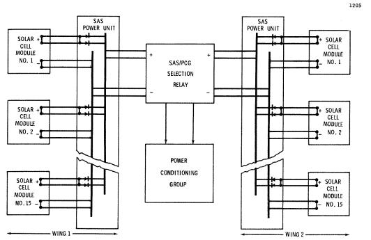
NOTE: FIFTEEN (15) SOLAR CELL MODULES FROM EACH WING ARE COLLECTED FOR A TOTAL OF 30 MODULES PER POWER GROUP. THIS ARRANGEMENT IS TYPICAL FOR EACH OF THE EIGHT POWER GROUPS
