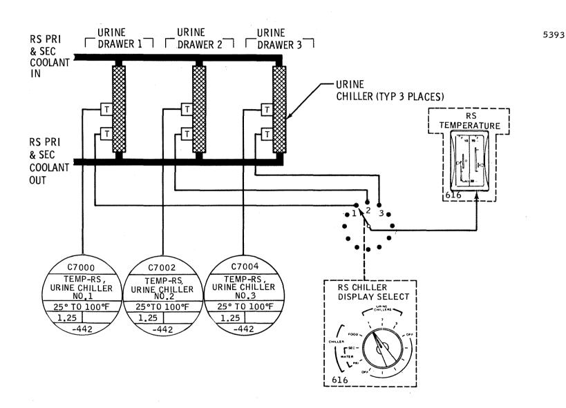
Figure 2.5.11-8 Urine Chiller -- Functional Diagram
