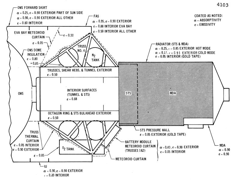
Figure 2.4.4-34 AM/MDA Thermal Coatings
