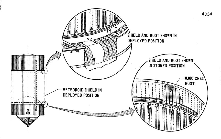
Figure 2.4.4-35 Meteoroid Shield Boot
