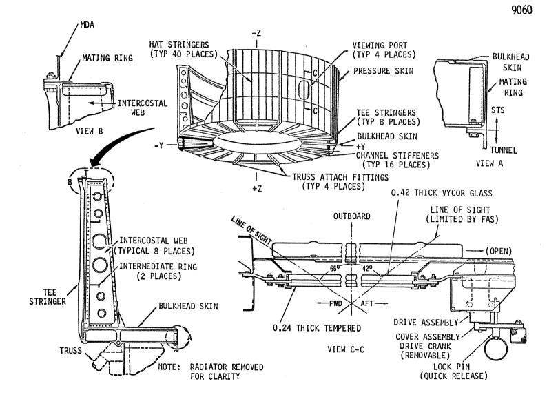
Figure 2.0.8-5 Structural Transition Section
