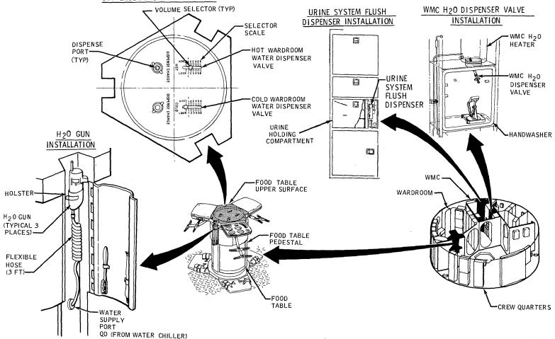
Figure 2.5.12-15 Water Management Dispensers -- Installation
