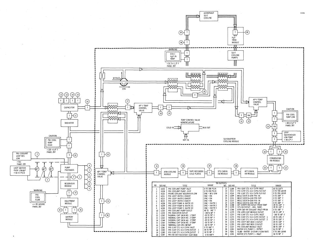
Figure 2.4.4-22 Primary Coolant Loop
