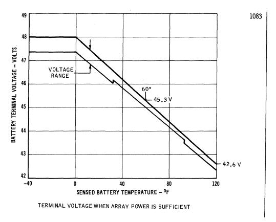
Figure 2.1.4-12 Battery Charger Voltage Limit Mode
