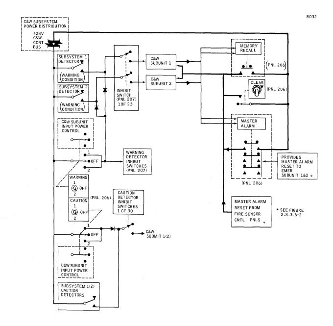
Figure 2.8.3-11 C&W Subsystem Control Signal Distribution
