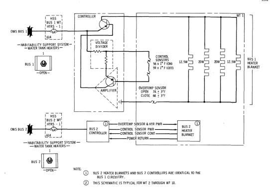
Figure 2.5.12-5 Typical Water Tank Heater Blanket -- Schematic
