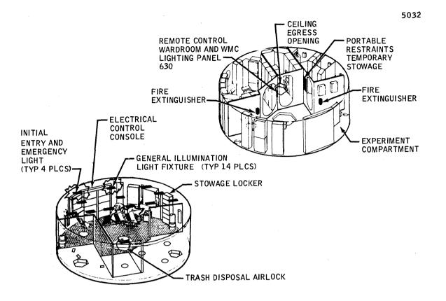
Figure 2.0.10-14 Experiment Compartment Arrangement
