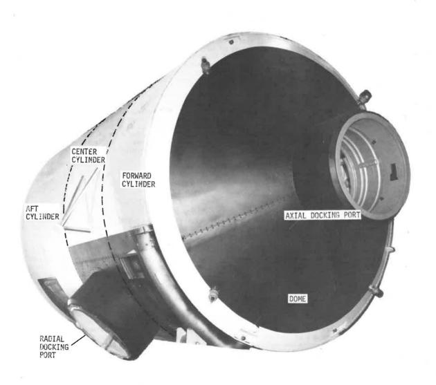
Figure 2.0.7-4 Structural Configuration
