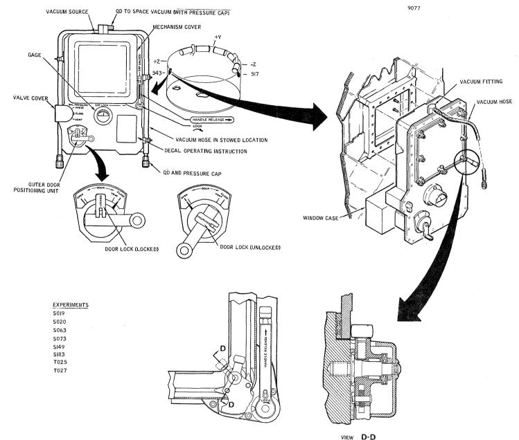
Figure 2.0.10-6 Scientific Airlock Configuration
