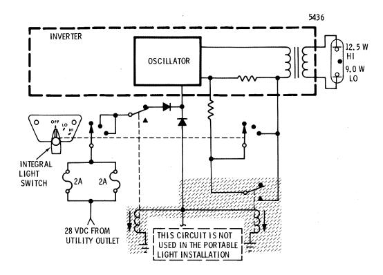
Figure 2.5.4-20 Floodlight Bulb -- Schematic (Portable Light Usage)
