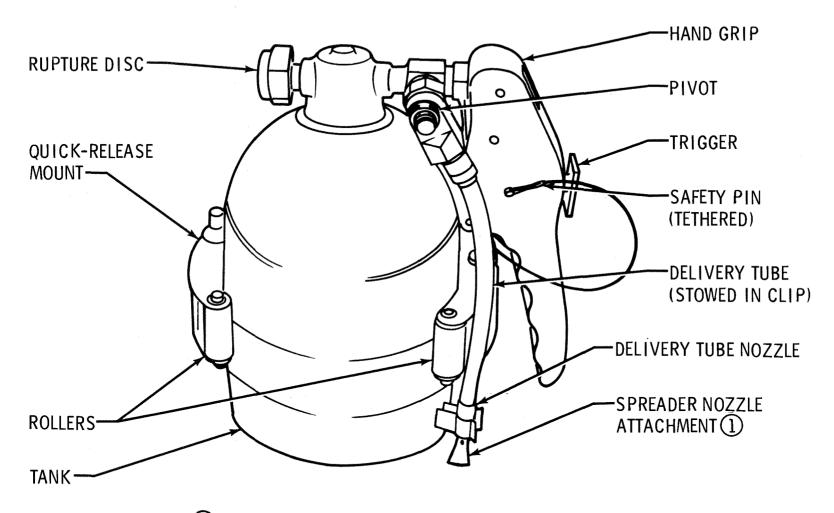
NOTE: 1 THE SPREADER NOZZLE CONNECTS TO THE DELIVERY TUBE NOZZLE WITH A QUICK RELEASE BALL-LOCK MECHANISM
