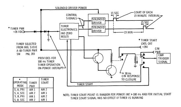
Figure 2.4.4-71 Molecular Sieve Cycle Timer
