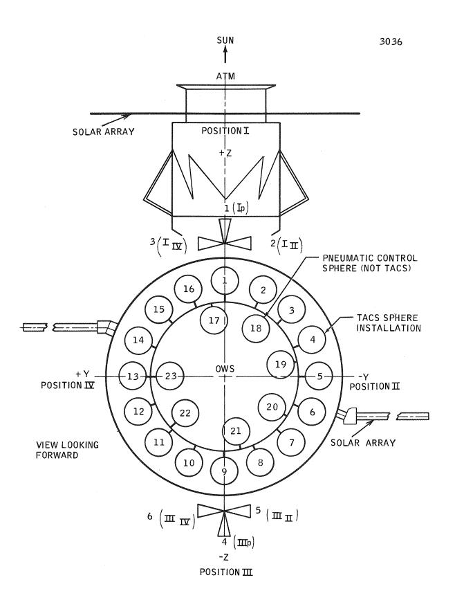
Figure 2.3.3-2 Thruster Module Orientation
