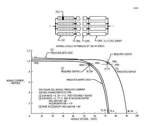
Figure 2.1.4-3 Solar Cell Module Characteristics
