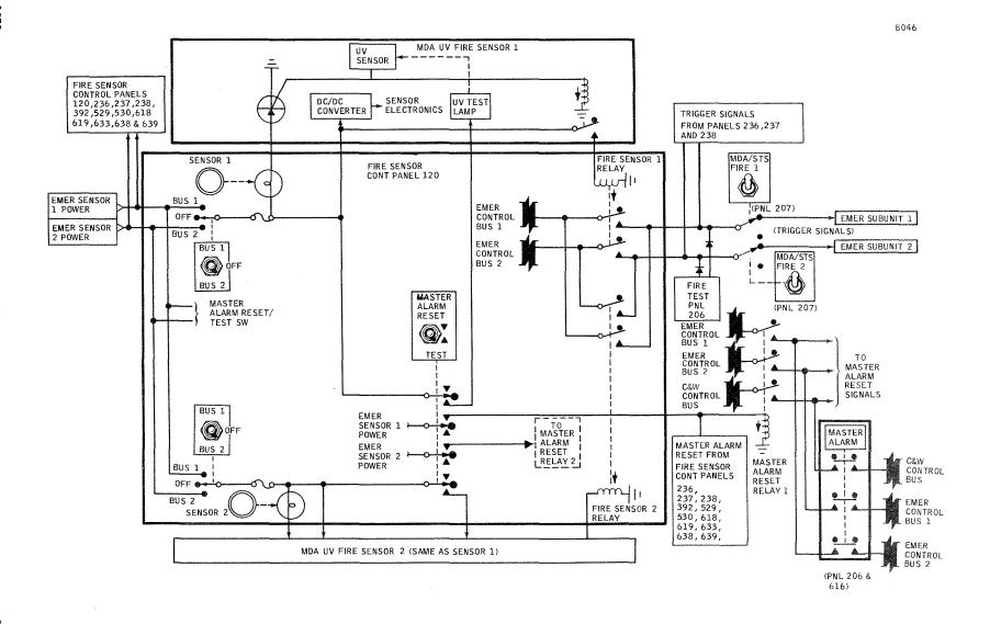
Figure 2.8.3-13 Fire Sensor Controls & Power Distribution (MDA/STS Group Typical)
