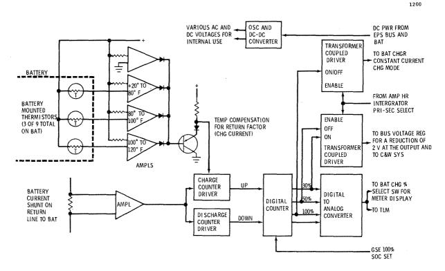
Figure 2.1.4-11 Amp-Hour Integrator Functional
