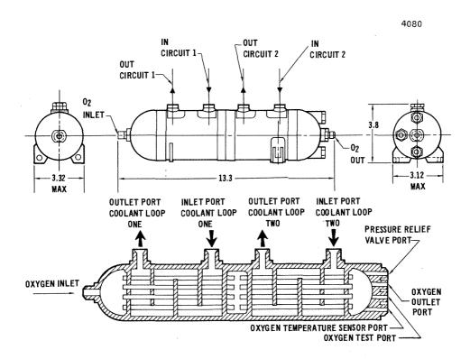
Figure 2.4.4-48 Oxygen Heat Exchanger
