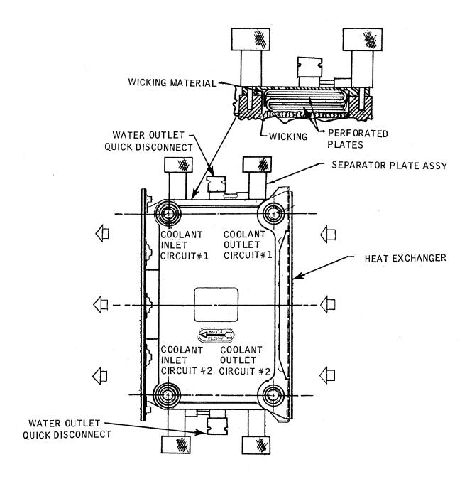
Figure 2.4.4-65 Condensing Heat Exchanger and Water Separator
