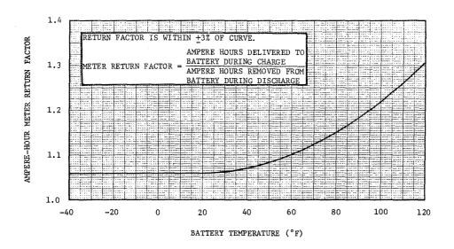
Figure 2.1.4-10 Ampere-Hour Integrator Return Factor
