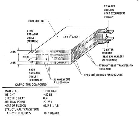
Figure 2.4.4-39 Thermal Capacitor
