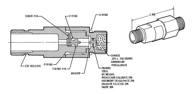
Figure 2.0.6-6 Pressure Cartridge
