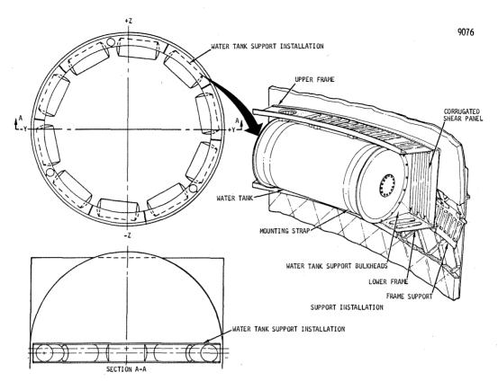
Figure 2.0.10-3 Water Tanks Configuration
