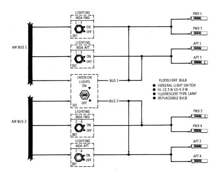
Figure 2.5.4-9 MDA Internal Lighting -- Functional Diagram
