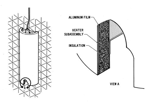
Figure 2.4.4-29 Radiant Heaters
