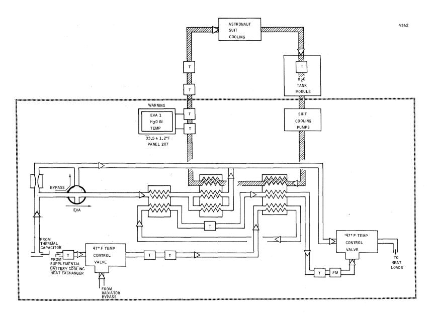
Figure 2.4.4-76 Suit Cooling System -- Coolant Loop Interface
