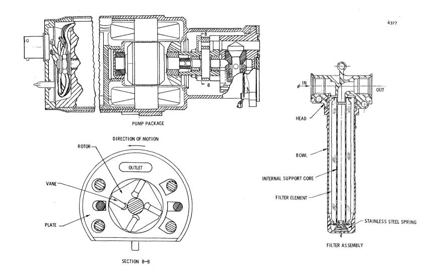
Figure 2.4.4-49 Water Pump and Filter
