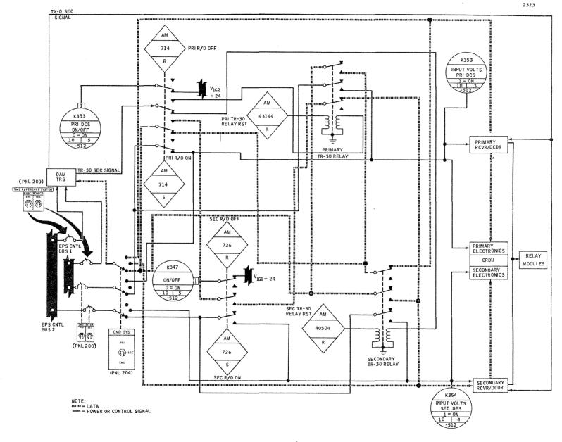
Figure 2.7.3-4 DCS Control -- Rcvr/Dcdr Control Switching Logic
