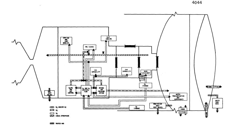
Figure 2.4.3-1 Pressurization and Gas Distribution
