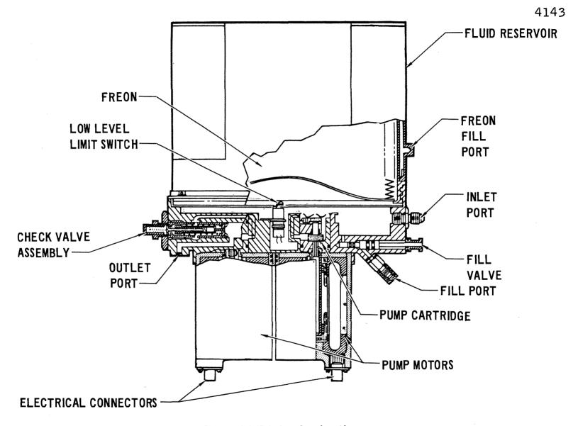
Figure 2.4.4-37 Coolant Pump Assembly
