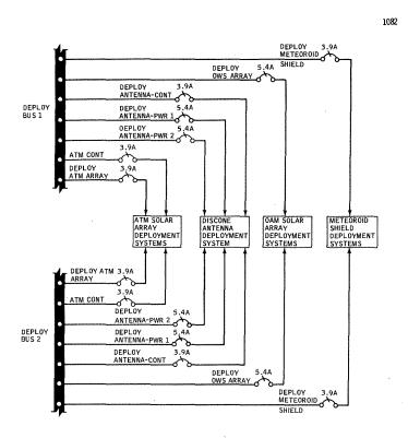
Figure 2.1.3-19 Deploy Bus Loads
