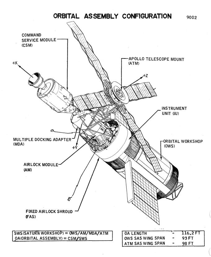
Figure 1.0-1 Orbital Assembly Configuration
