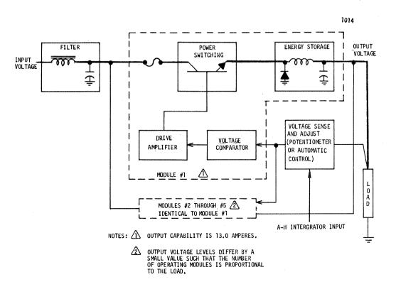
Figure 2.1.4-14 Bus Voltage Regulator Power Diagram
