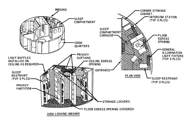
Figure 2.0.10-13 Sleep Compartment Arrangement
