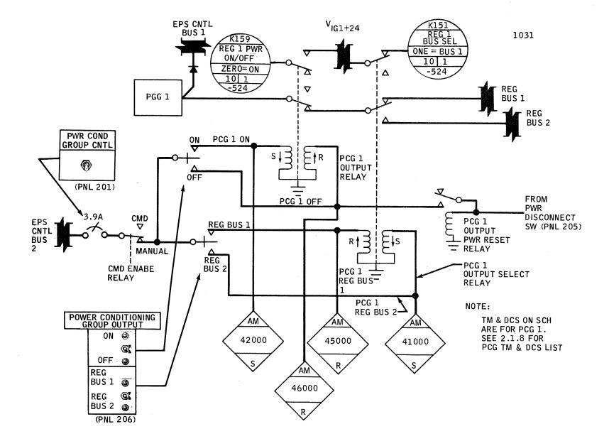
Figure 2.1.3-11 PCG Output Schematic
