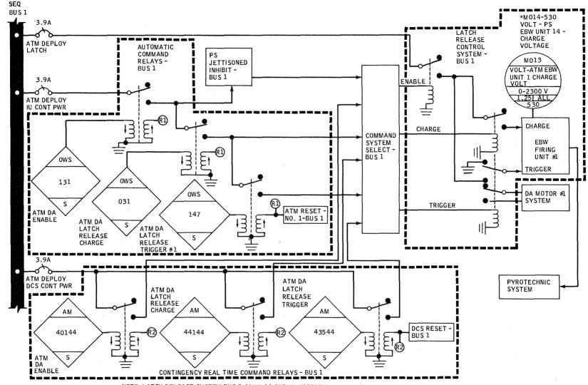
NOTE: LATCH RELEASE SYSTEM BUS 2 SAME AS SHOWN EXCEPT WITH (176) ATM DA LATCH RELEASE TRIGGER #2 (057) AND ATM DA RESET #2 (176)
