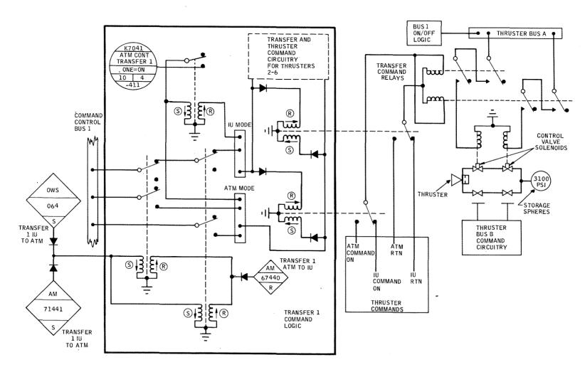
Figure 2.3.3-8 Transfer and Thruster Command -- Schematic
