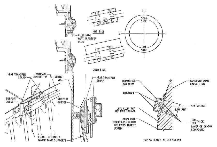
Figure 2.4.4-25 Heat Pipe Installation -- OWS Wall
