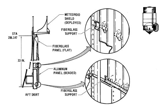
Figure 2.4.4-36 Forward and Aft Thermal Shield
