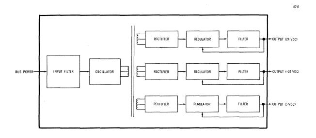
Figure 2.6.4-3 AM Panel Indicator DC-DC Converter
