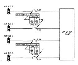
Figure 2.2.3-2 Audio Subsystem Power Distribution
