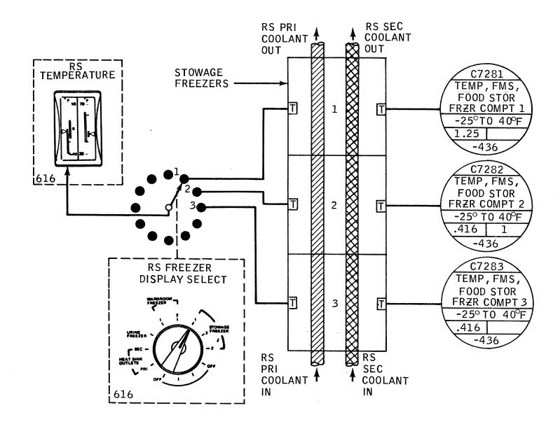
Figure 2.5.10-4 Stowage Freezers -- Functional Diagram
