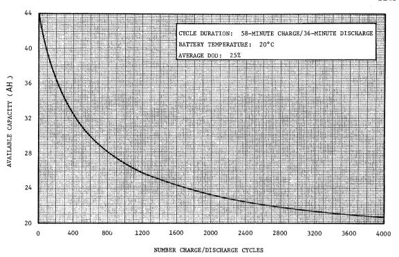
Figure 2.1.4-13 AM Battery Degradation
