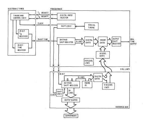
Figure 2.6.4-17 Digital Time Channels
