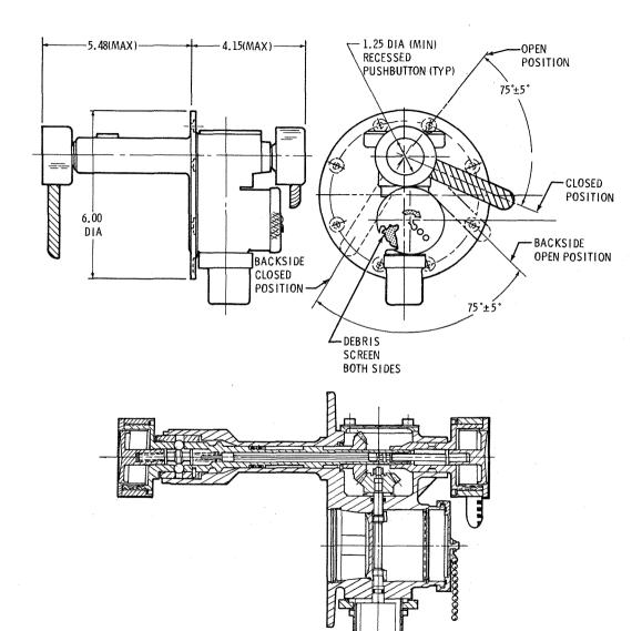
Figure 2.4.4-13 Pressure Equalization Valve
