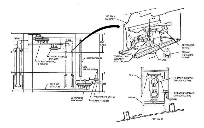
Figure 2.0.10-26 SAS Beam Fairing Release System
