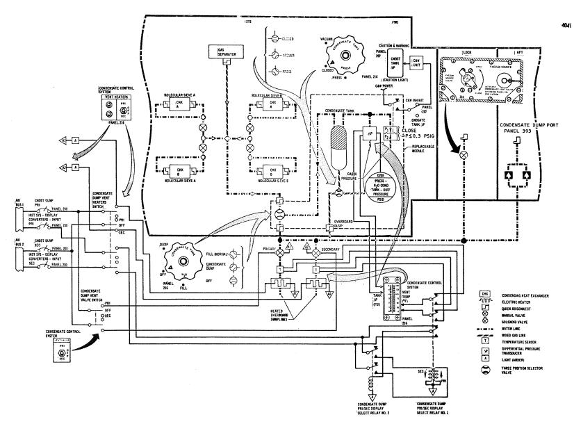
Figure 2.4.4-58 Condensate Collection and Removal
