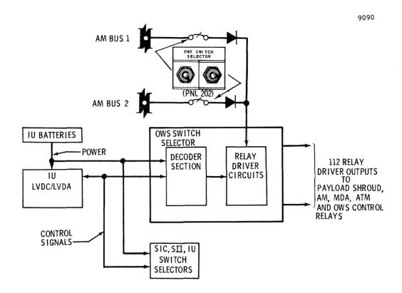
Figure 2.11.3-2 OWS Switch Selector Power
