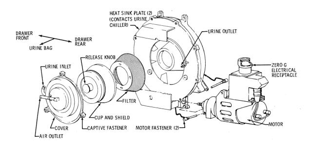
Figure 2.5.11-10 Urine Separator -- Exploded View
