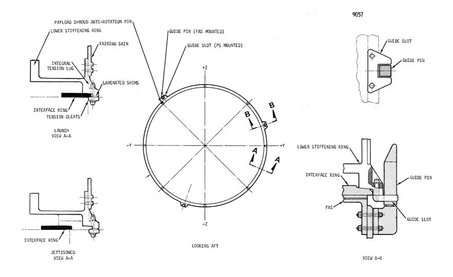
Figure 2.0.3-4 Payload Shroud to FAS Interface
