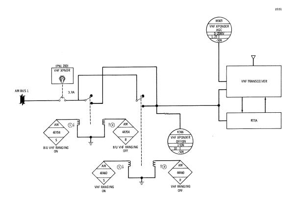
Figure 2.2.3-5 Ranging Subsystem Configuration
