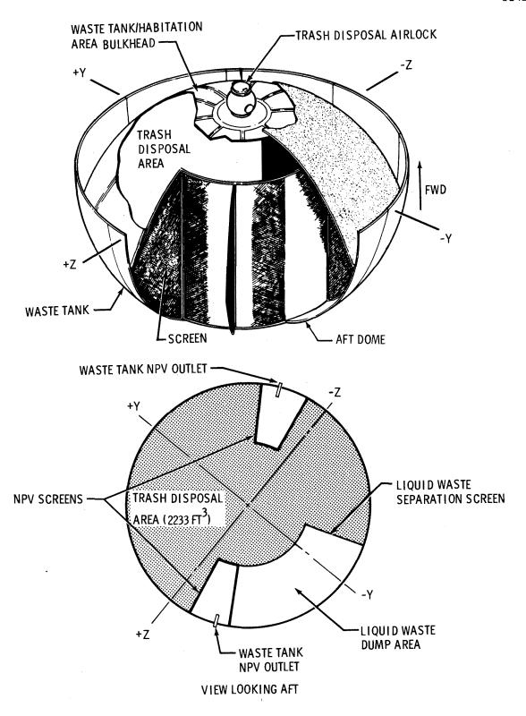
Figure 2.5.9-5 Waste Tank Trash Disposal
