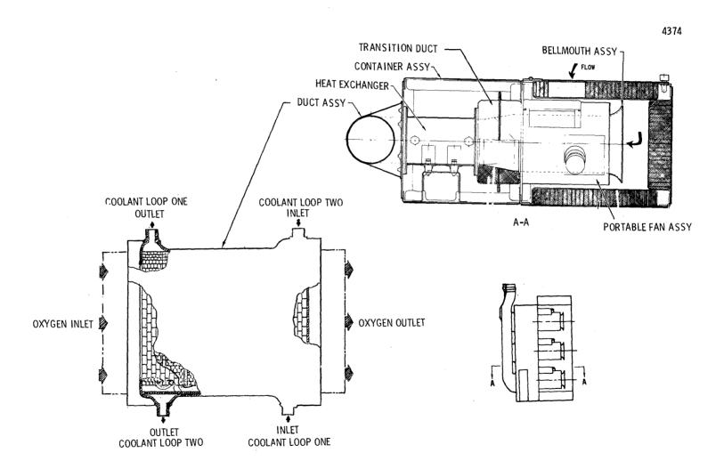
Figure 2.4.4-64 Cabin Heat Exchanger
