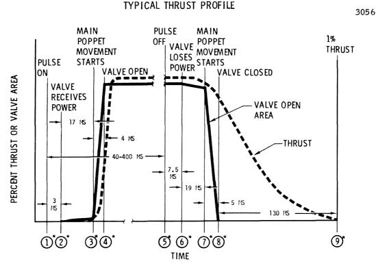
Figure 2.3.6-2 Typical Thrust Profile
