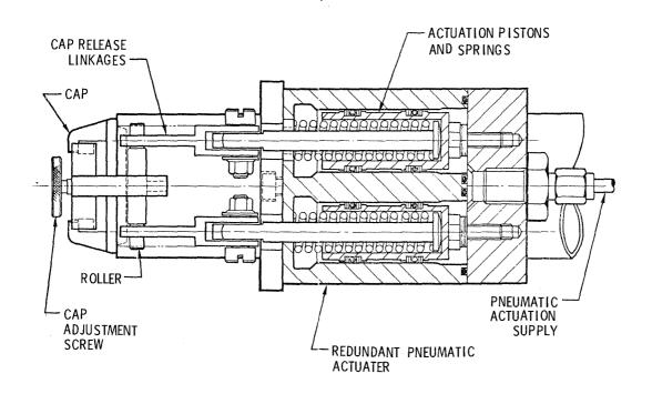
Figure 2.4.4-10 Waste Tank NPV and Cap Release
