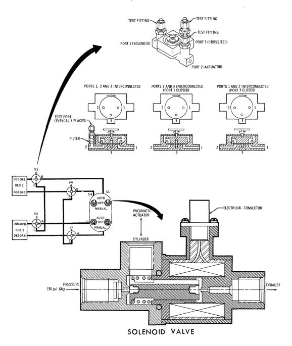
Figure 2.4.4-70 Molecular Sieve Solenoid & Manual Interconnect Valves
