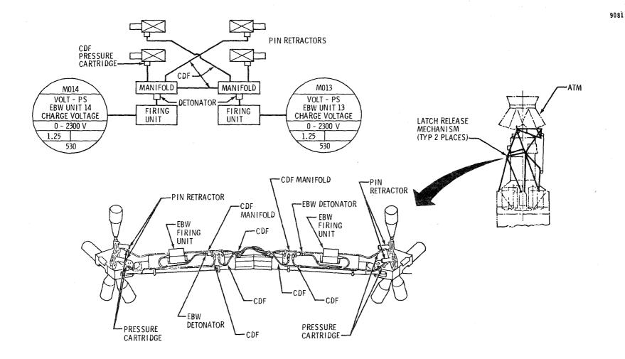
Figure 2.0.6-4 ATM Deployment Release Mechanism
