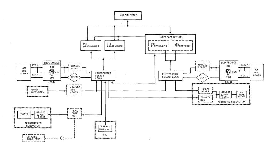
Figure 2.6.3-3 PCM Subsystem
