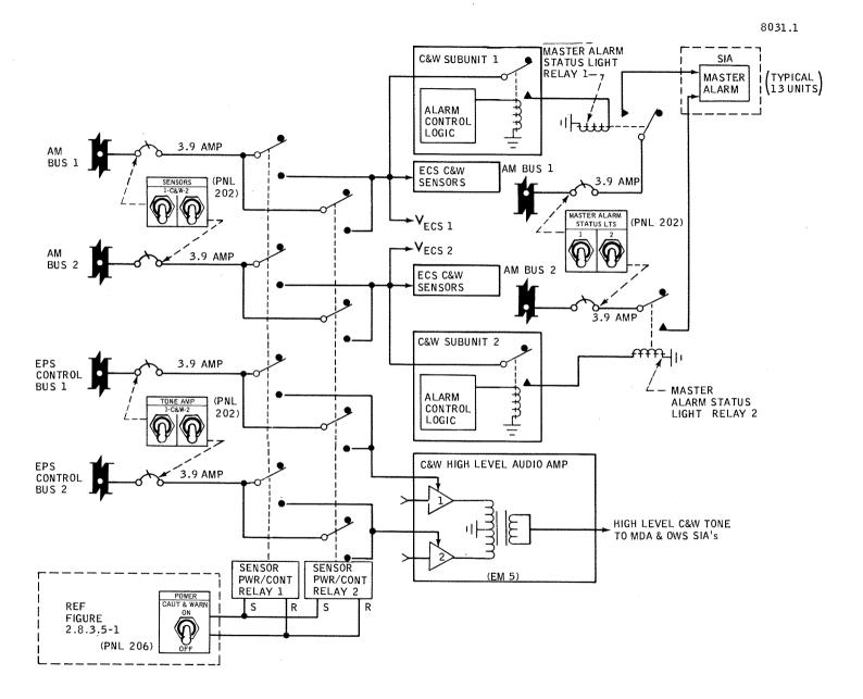
Figure 2.8.3-10 C&W Subsystem Power Distribution (Sheet 2)
