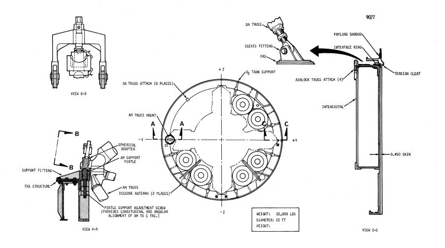
Figure 2.0.9-1 Fixed Airlock Shroud
