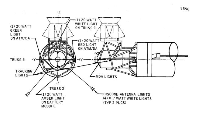
Figure 2.9-1 Tracking and Docking Lights
