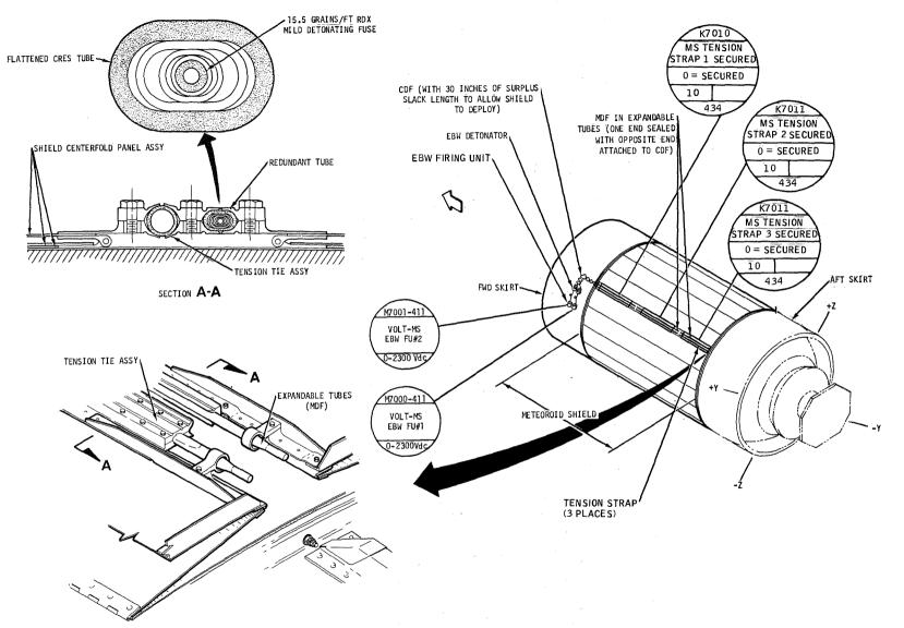
Figure 2.0.10-35 Meteoroid Shield Deployment Ordnance System
