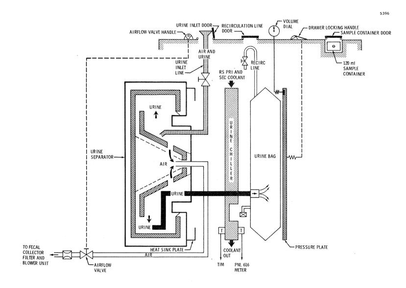
Figure 2.5.11-7 Typical Urine Drawer -- Schematic
