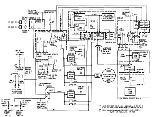
Figure 2.8.2-2 CSM Caution/Warning Subsystem
