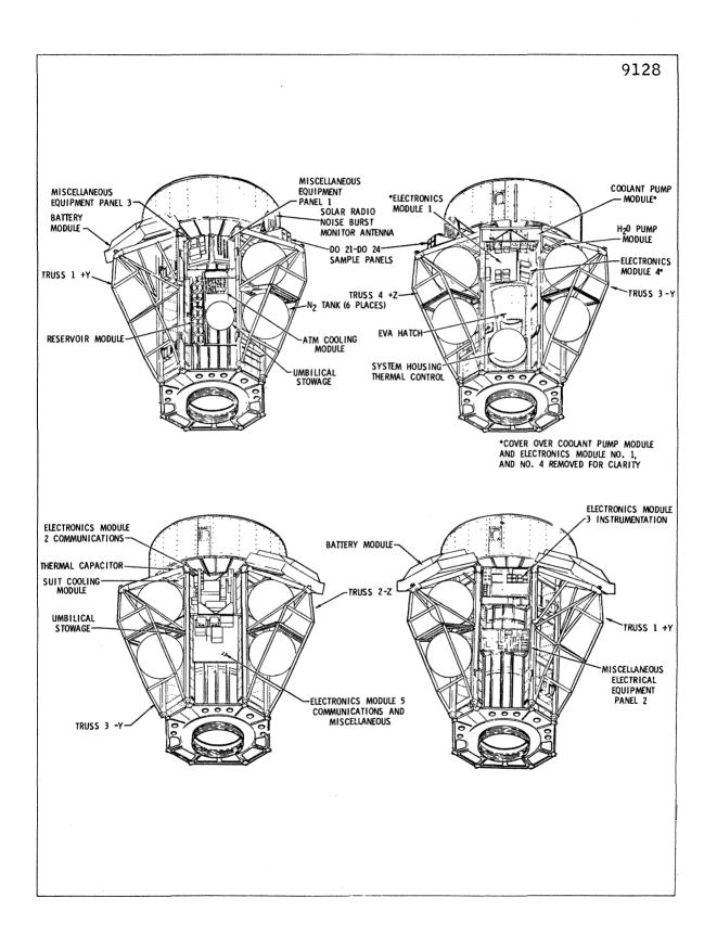
Figure 2.0.8-3 AM External Configuration
