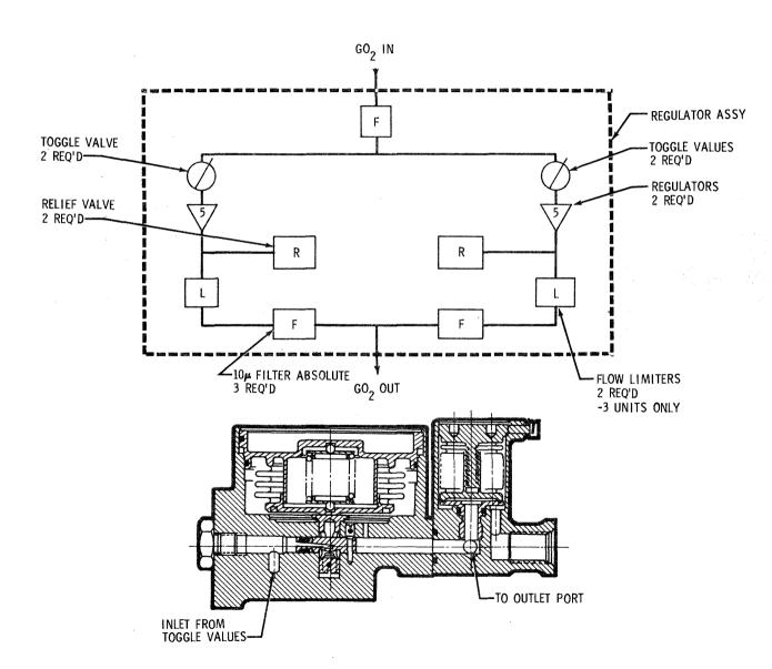
Figure 2.4.4-17 Water Reservoir Pressure Regulator
