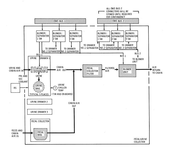
Figure 2.5.11-5 Fecal/Urine Collector -- Block Diagram
