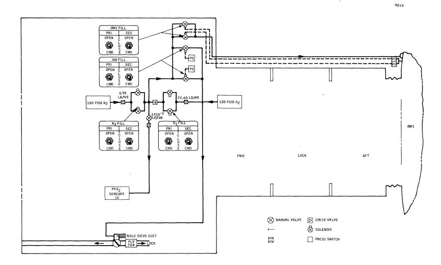
Figure 2.4.4-6 AM/MDA and OWS Pressurization
