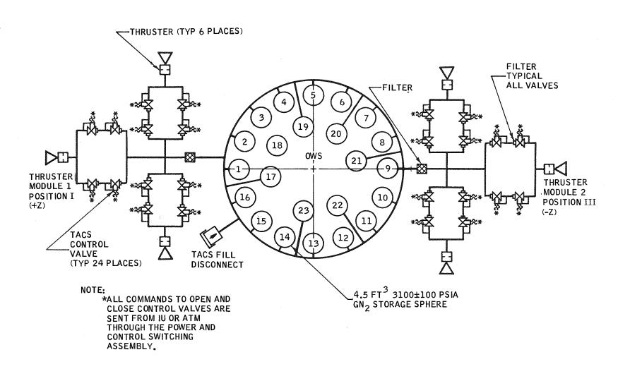
Figure 2.3.3-3 TACS Propellant Supply/Distribution
