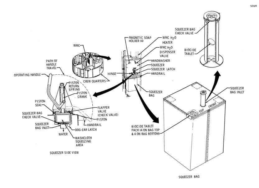
Figure 2.5.12-17 Partial Body Cleansing Facilities - Handwasher
