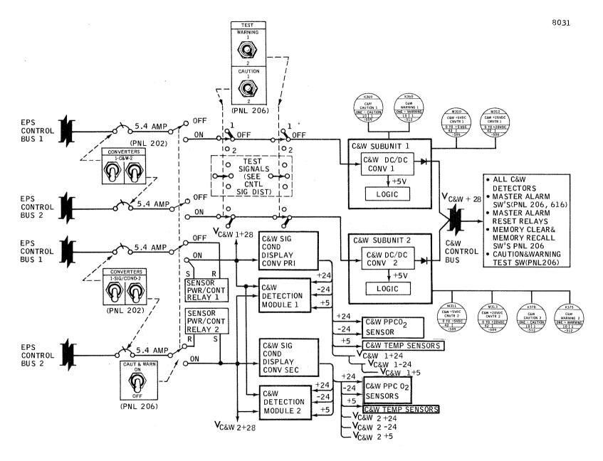
Figure 2.8.3-10 C&W Subsystem Power Distribution (Sheet 1)
