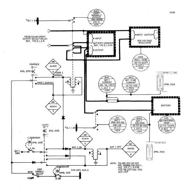
Figure 2.1.3-7 Simplified PCG Schematic
