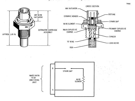
Figure 2.0.3-8 EBW Detonator
