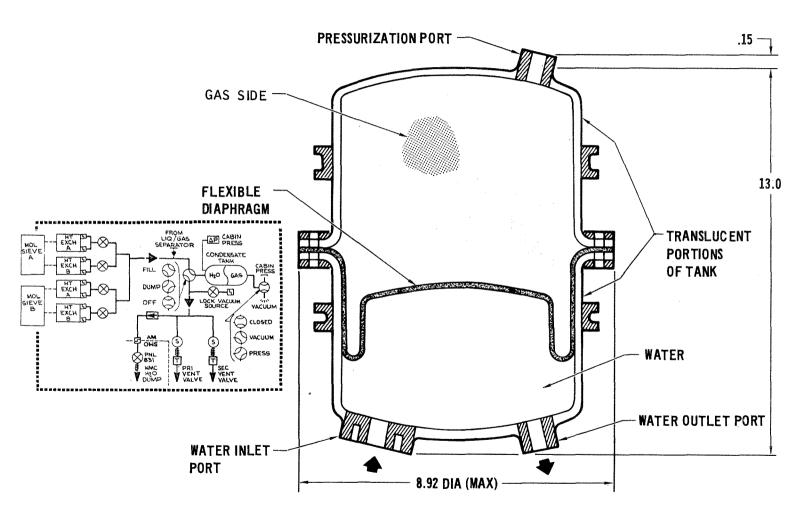
Figure 2.4.4-67 Condensate Tank Assembly
