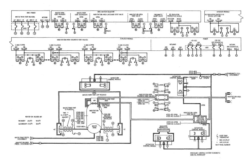
Figure 2.4.4-2 Habitation Area and Waste Tank Venting
