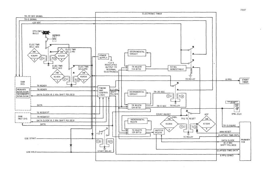
Figure 2.7.4-4 Electronic Timer Operation
