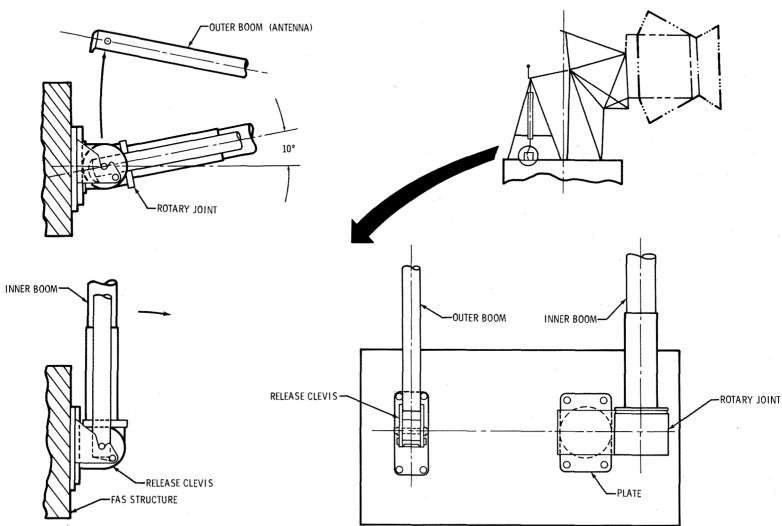
Figure 2.0.4-4 Discone Antenna Rotation Assembly
