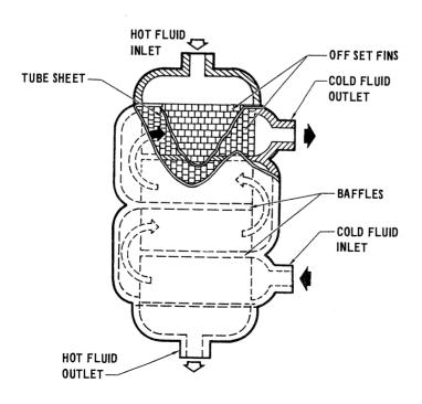
Figure 2.4.4-45 Regenerative-Type Heat Exchanger
