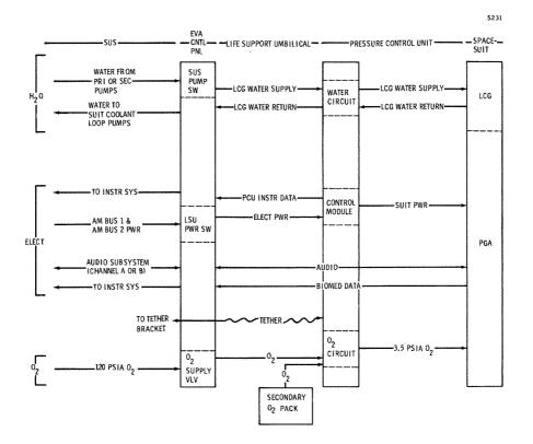
Figure 2.5.7-7 Life Support Systems - Functional Diagram
