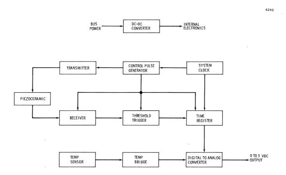
Figure 2.6.4-9 Water Level Transducer
