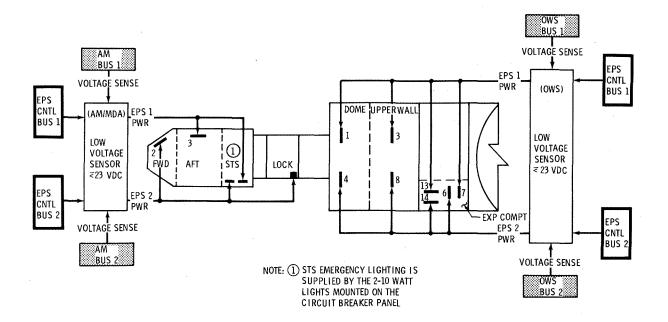
Figure 2.5.4-17 Emergency Lighting -- Functional Diagram
