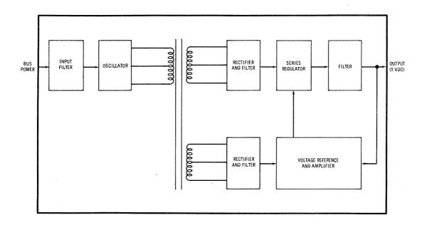
Figure 2.6.4-4 OWS DC-DC Converter
