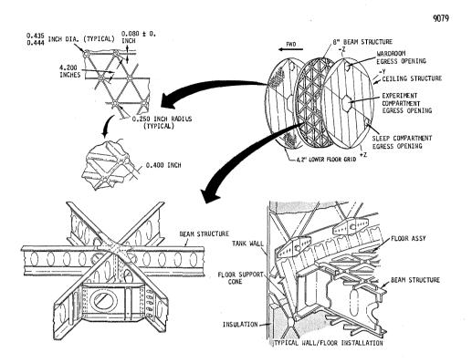
Figure 2.0.10-5 Forward Compartment Floor Structure
