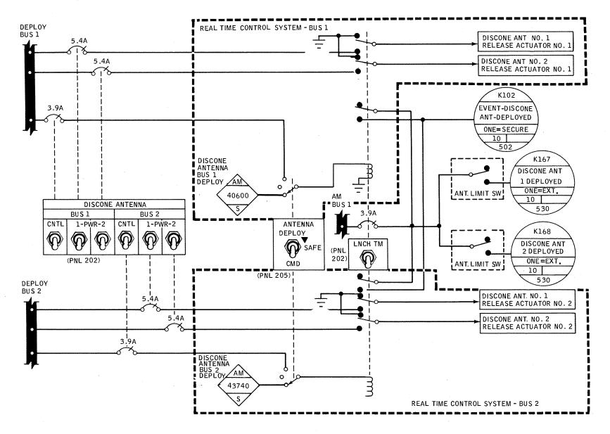
Figure 2.0.4-5 Discone Antenna Deployment
