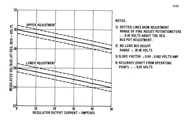
Figure 2.1.4-15 Bus Voltage Regulator Output Adjustment Characteristics
