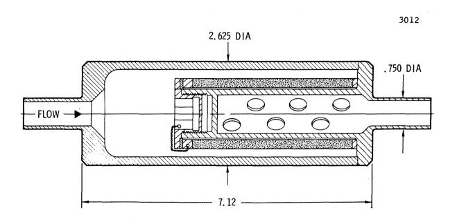
Figure 2.3.4-6 Thruster Supply Line Filter
