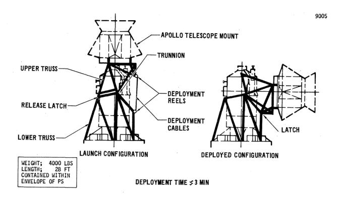
Figure 2.0.6-1 ATM Deployment Assembly
