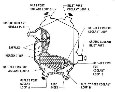
Figure 2.4.4-40 Ground Cooling Heat Exchanger
