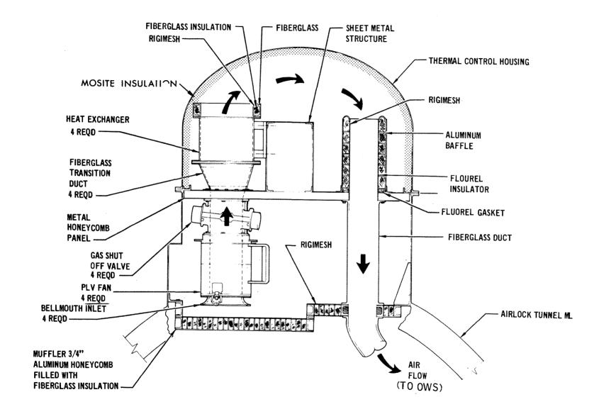
Figure 2.4.4-53 OWS Cooling Module
