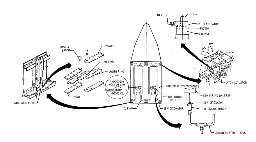
Figure 2.0.3-5 Payload Shroud Latch Actuator System
