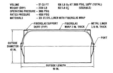
Figure 2.4.4-4 02/N2 Tank Arrangement
