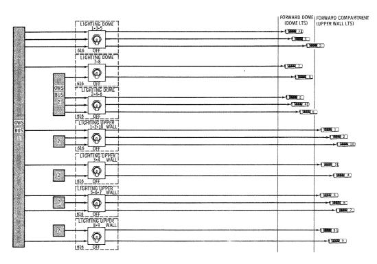
Figure 2.5.4-14 OWS Forward Area Lighting -- Functional Diagram
