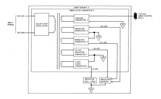
Figure 2.8.4-6 Emergency Subunits DC/DC Converters
