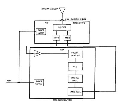
Figure 2.2.4-5 Ranging Subsystem Operation
