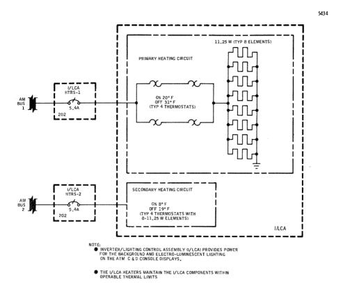
Figure 2.5.4-11 I/LCA Heater -- Schematic
