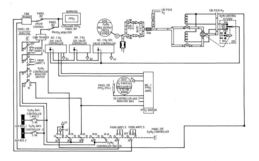
Figure 2.4.4-19 PPO2 Sensor, Amplifier, Controller
