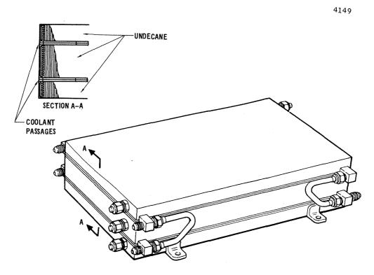
Figure 2.4.4-82 Thermal Capacitor - Refrigeration System
