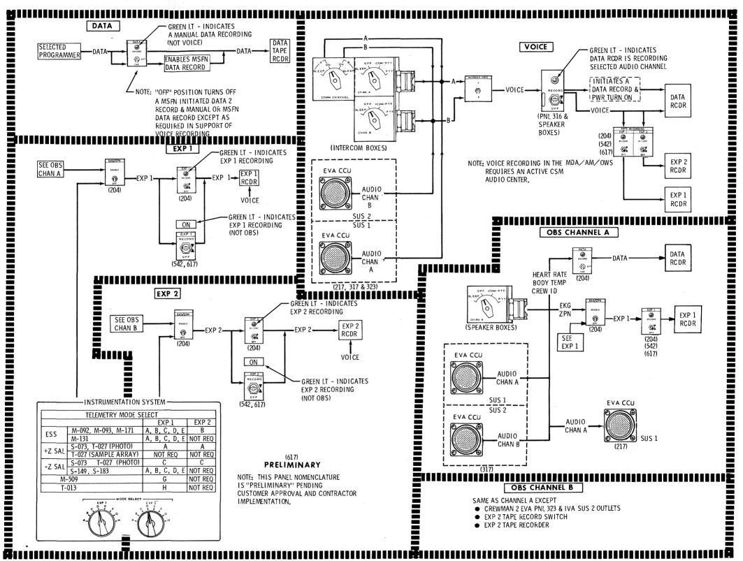
Figure 2.6.3-5 Tape Recording Flow Diagram
