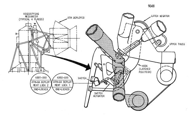
Figure 2.0.6-13 DA Latching Mechanism
