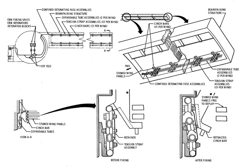
Figure 2.0.10-29 SAS Wing Panel Release System
