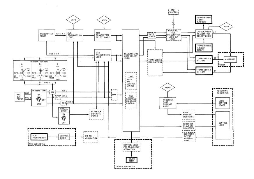
Figure 2.6.3-6 Transmission Subsystem
