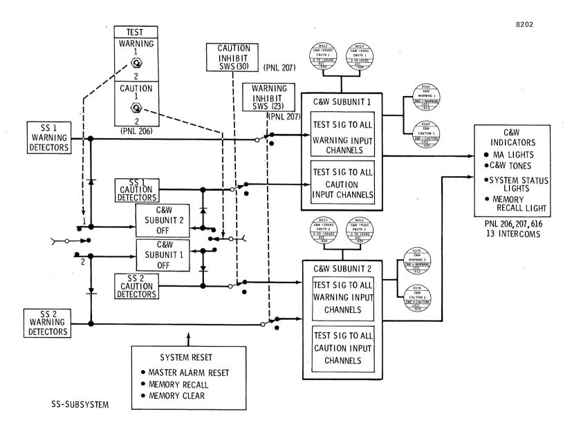
Figure 2.8.3-4 C&W Subsystem Self-Test
