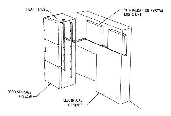
Figure 2.4.4-26 Heat Pipe Installation -- Food Freezer
