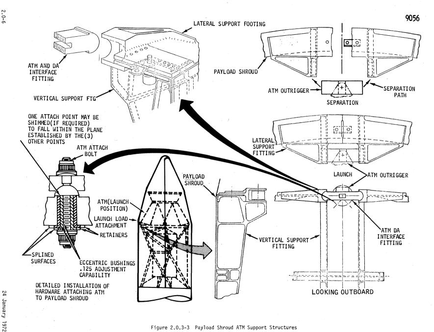
Figure 2.0.3-3 Payload Shroud ATM Support Structures
