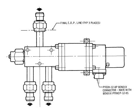
Figure 2.4.4-50 Heat Exchanger Coolant Flow Bypass Valve
