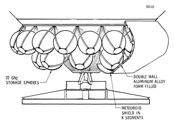
Figure 2.3.4-4 Spheres and Meteoroid Shield
