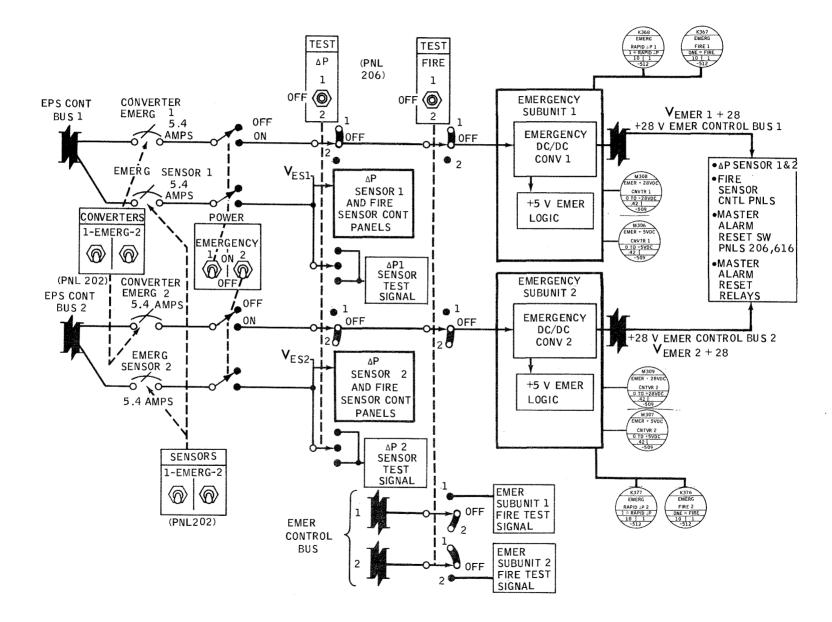
Figure 2.8.3-12 Emergency Subsystem Power Distribution
