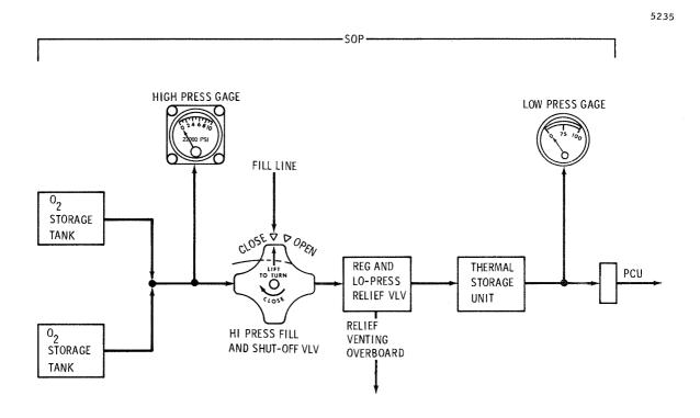
Figure 2.5.7-8 ALSA SOP -- Functional Diagram
