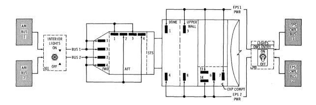
Figure 2.5.4-16 Entry Lighting -- Functional Diagram
