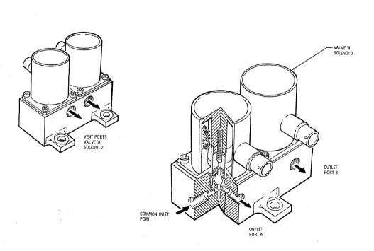
Figure 2.4.4-8 Actuation Control Module
