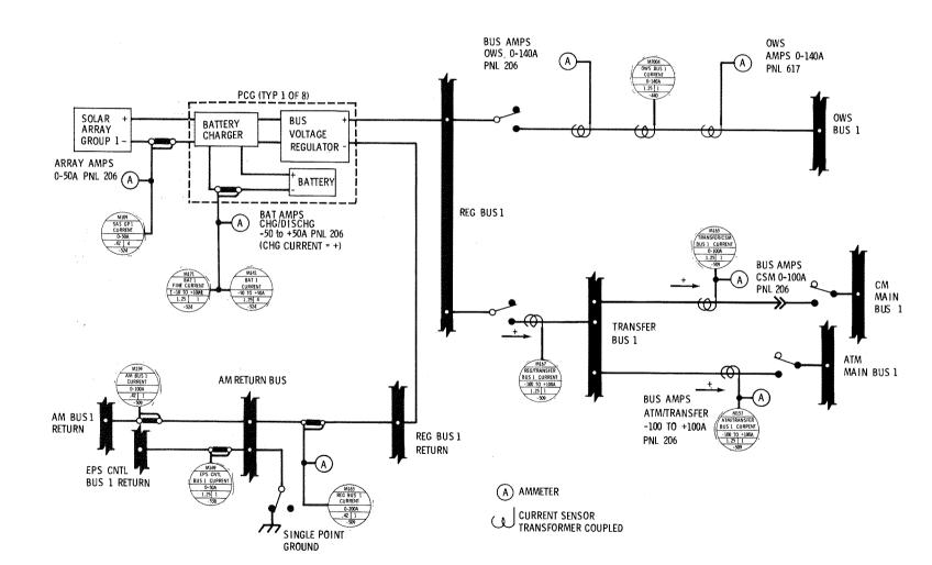
Figure 2.1.3-12 Typical Shunt/Current Sensor Arrangement
