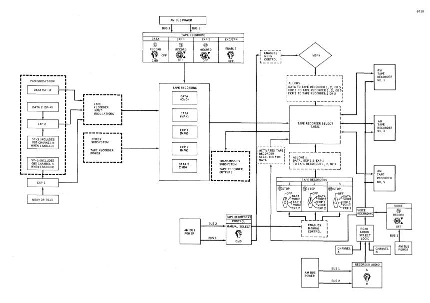
Figure 2.6.3-4 Recording Subsystem
