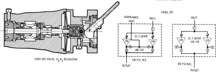
Figure 2.4.4-14 Pressure Regulator Assembly
