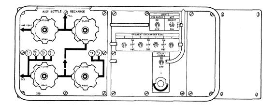
Figure 2.4.4-18 M509 Recharge Station (Panel 390)
