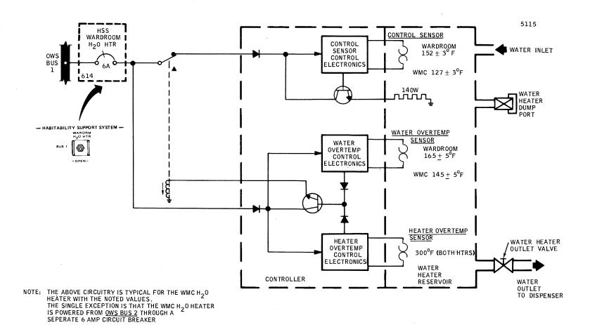
Figure 2.5.12-12 Water Heater -- Functional Diagram
