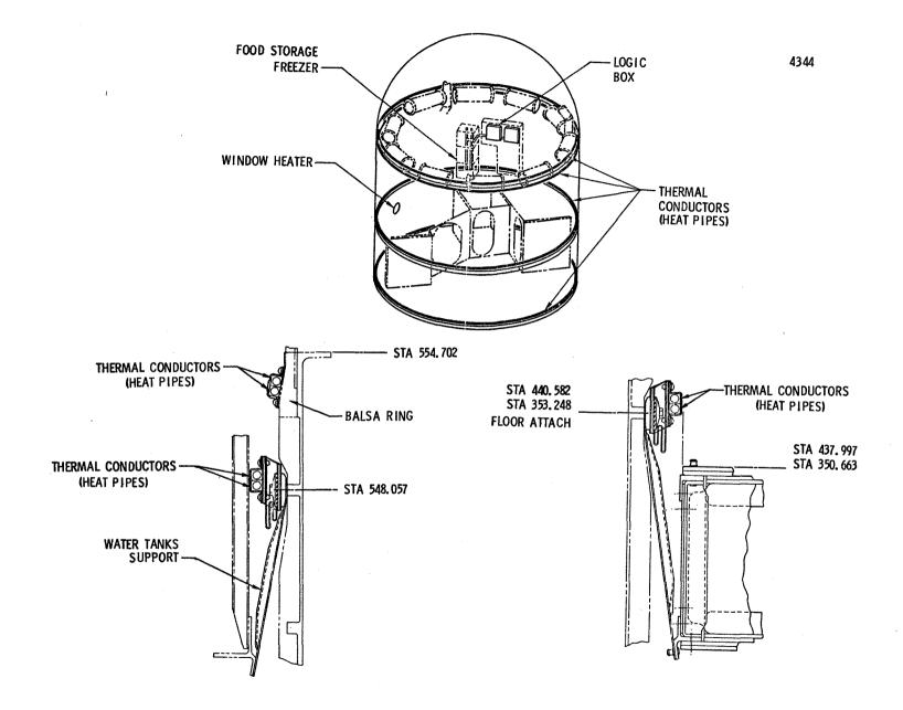
Figure 2.4.4-24 Heat Pipe Locations
