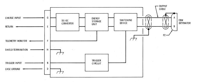
Figure 2.0.3-7 EBW Firing Unit
