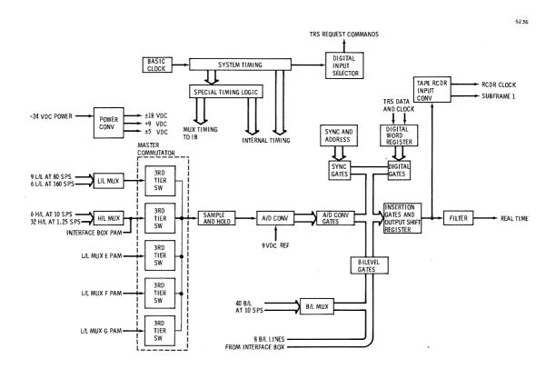
Figure 2.6.4-12 Programmer Block Diagram
