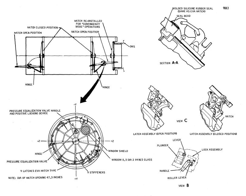
Figure 2.0.8-11 Interior Hatches
