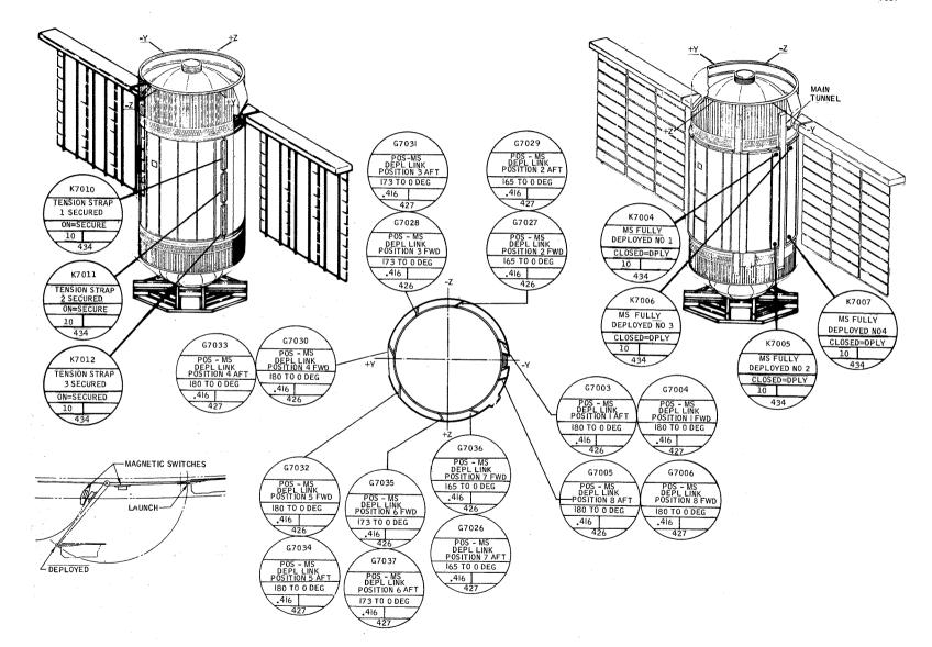
Figure 2.0.10-37 Meteoroid Shield Deployment Instrumentation
