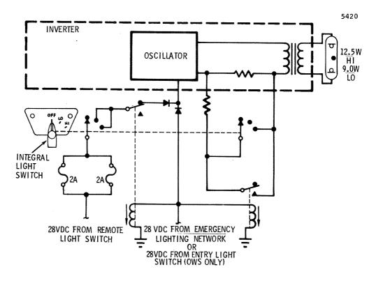
Figure 2.5.4-10 Floodlight Bulb -- Schematic
