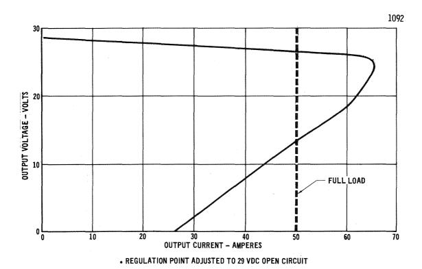
Figure 2.1.4-16 Bus Voltage Regulator V-I Characteristics
