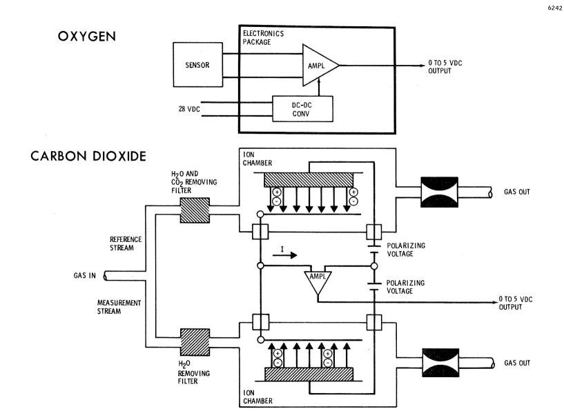
Figure 2.6.4-7 Partial Pressure Transducers
