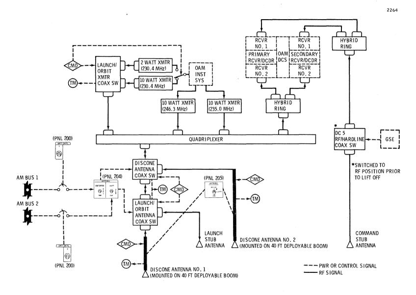
Figure 2.2.3-6 RF Subsystem Configuration
