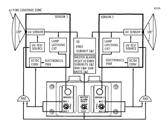
Figure 2.8.3-8 Fire Sensor Test
