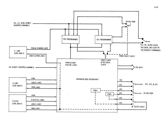
Figure 2.6.4-10 Multiplexing/Encoding Components Signal Flow
