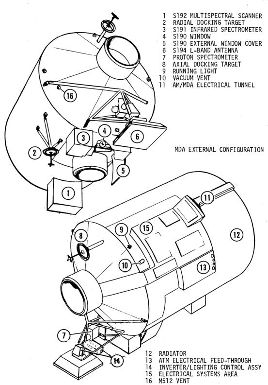
Figure 2.0.7-1 MDA External Configuration
