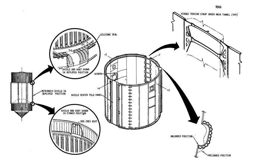
Figure 2.0.10-33 Meteoroid Shield Configuration
