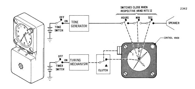
Figure 2.7.4-8 Portable Timer Operation
