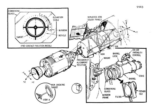
Figure 2.9-2 Crewman Optical Alignment Sight (COAS)
