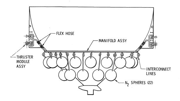
Figure 2.3.4-5 Storage Sphere Installation
