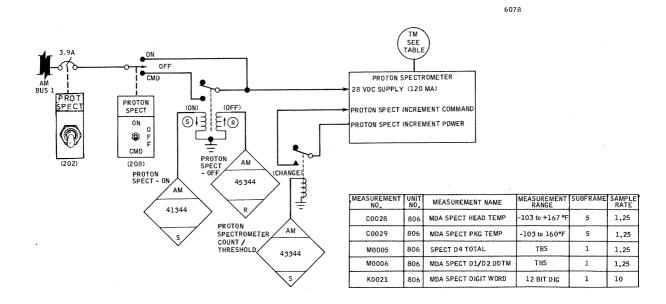
Figure 2.6.3-10 Proton Spectrometer
