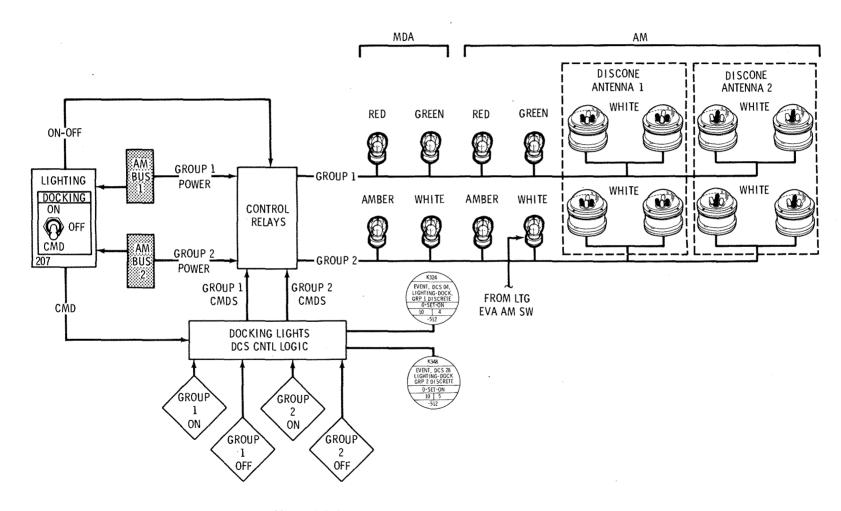
Figure 2.5.4-4 Docking Lights -- Functional Diagram
