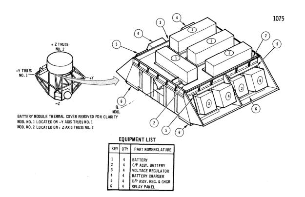
Figure 2.1.4-8 Typical Battery Module
