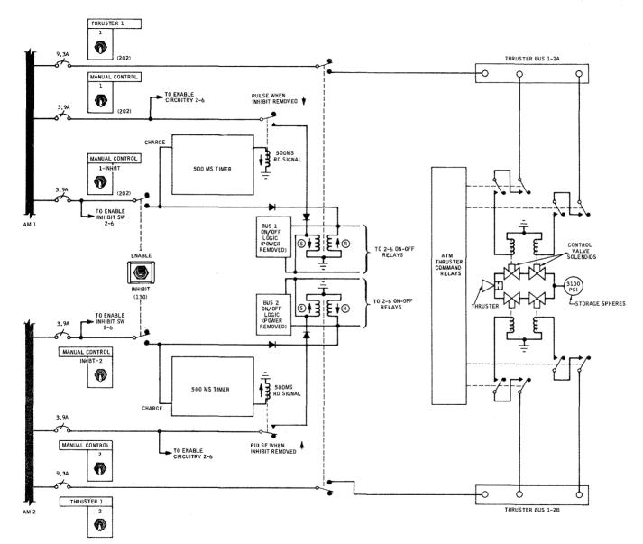
Figure 2.3.3-10 Manual Inhibit Control
