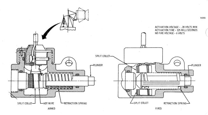
Figure 2.0.4-6 Release Actuator
