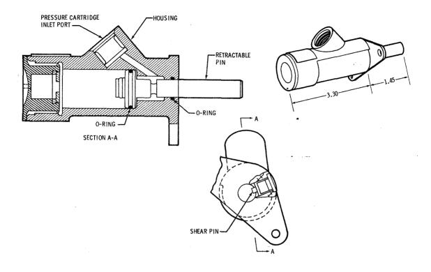
Figure 2.0.6-5 Pin Retractor
