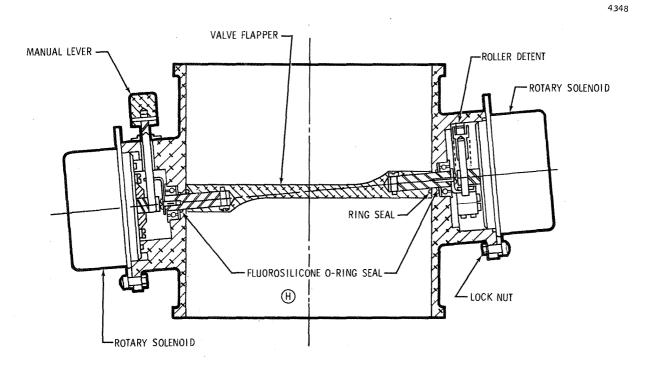
Figure 2.4.4-63 Gas Circulation Shutoff Valve
