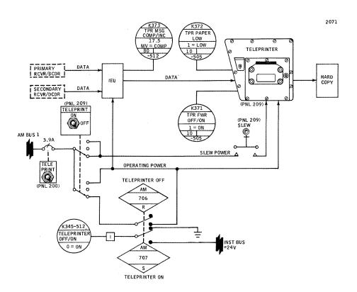
Figure 2.2.3-4 Teleprinting Subsystem Configuration
