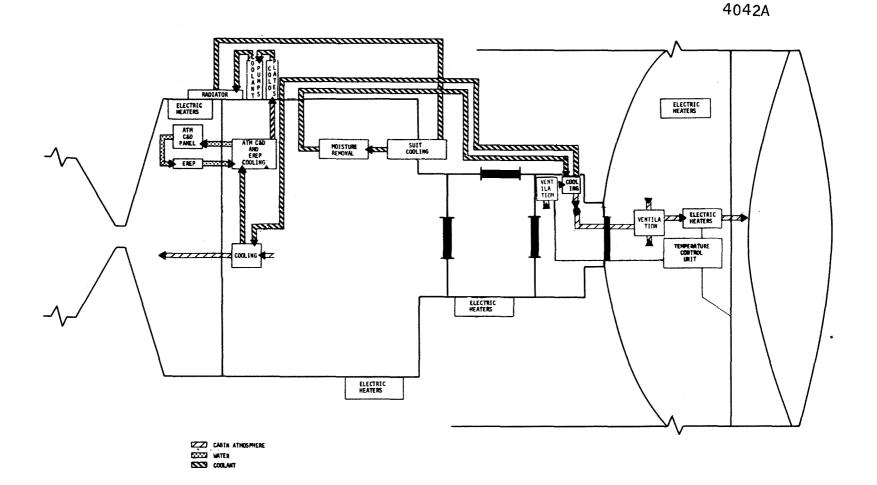
Figure 2.4.3-2 Thermal Control
