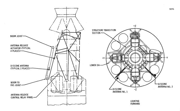
Figure 2.0.4-2 Discone Antenna Booms -- Configuration
