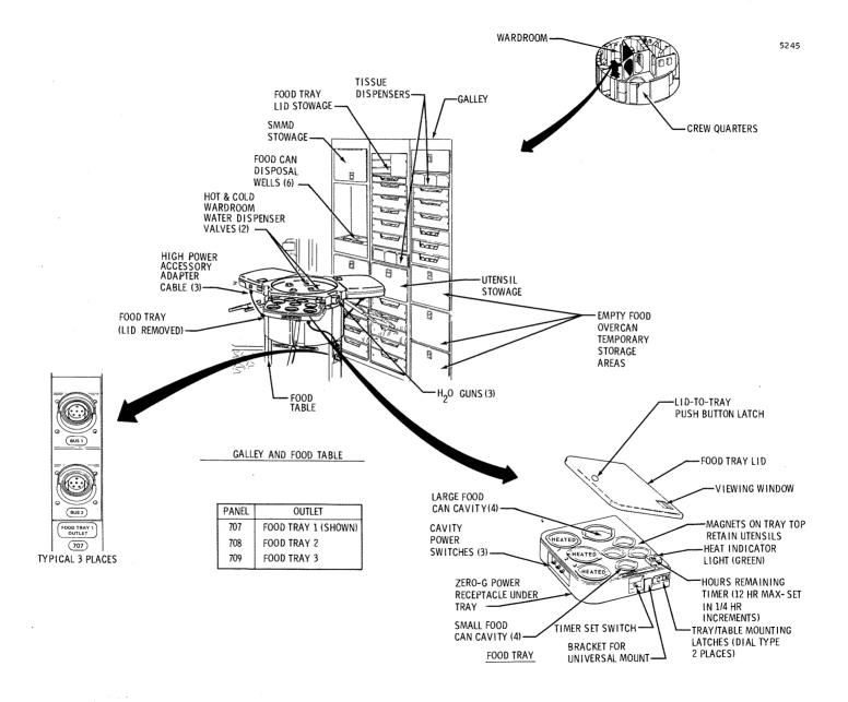
Figure 2.5.10-6 Food Preparation and Consumption Equipment
