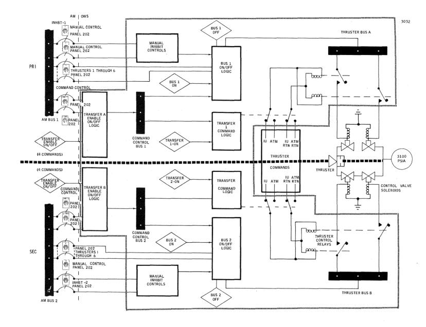
Figure 2.3.3-4 Single Thruster Control -- Schematic
