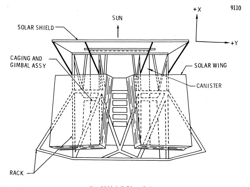
Figure 2.0.5-1 Apollo Telescope Mount
