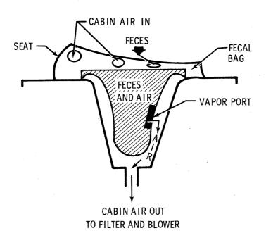
Figure 2.5.11-2 Fecal Collector -- Functional Diagram
