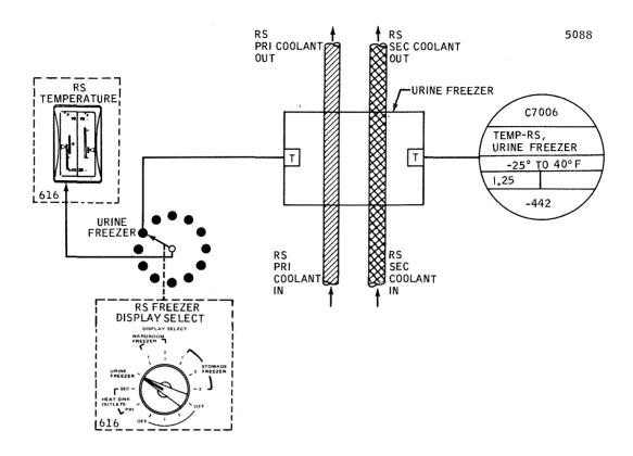
Figure 2.5.11-13 Urine Freezer -- Functional Diagram
