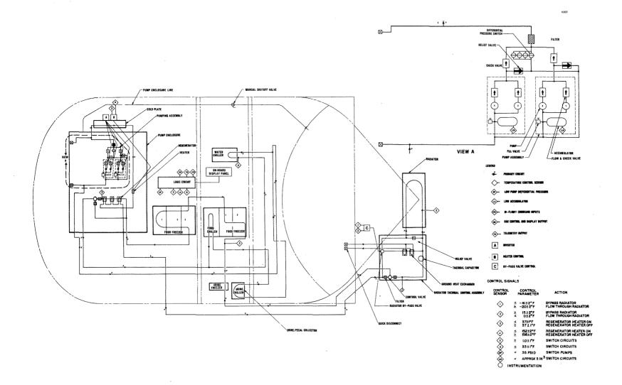
Figure 2.4.4-80 Refrigeration System Coolant Loop
