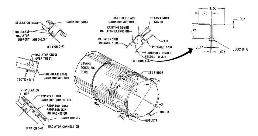
Figure 2.4.4-42 Radiator Configuration
