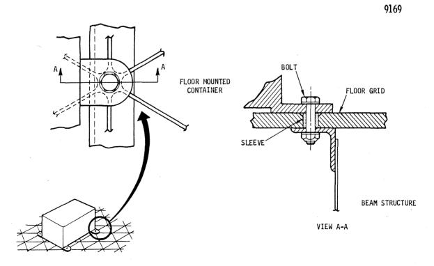
Figure 2.0.10-4 Container Floor Mounting
