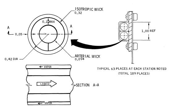
Figure 2.4.4-27 Heat Pipe Section
