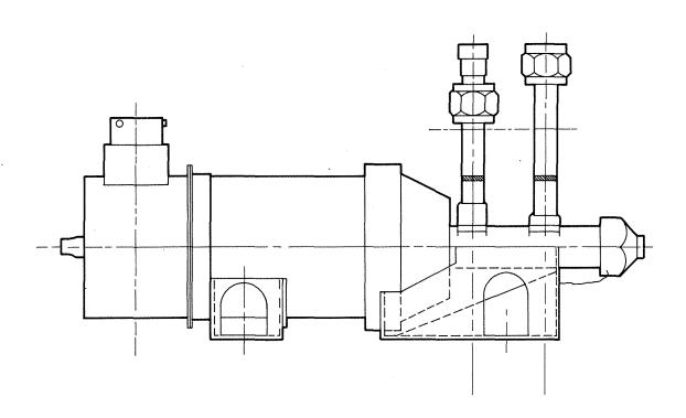
Figure 2.4.4-15 Latching Solenoid Valve
