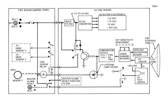
Figure 2.8.4-2 UV Fire Sensor
