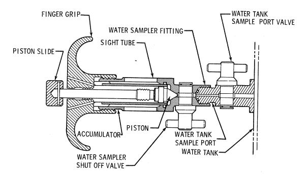
Figure 2.5.12-19 Water Sampler
