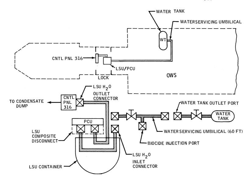
Figure 2.5.7-10 LSU/PCU Servicing -- Functional Diagram
