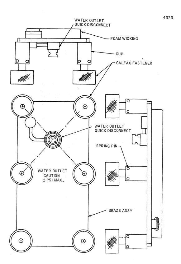
Figure 2.4.4-66 Water Separator Plate Assembly
