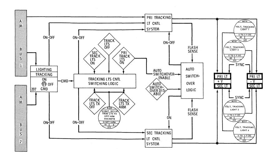
Figure 2.5.4-2 Tracking Lights -- Functional Diagram
