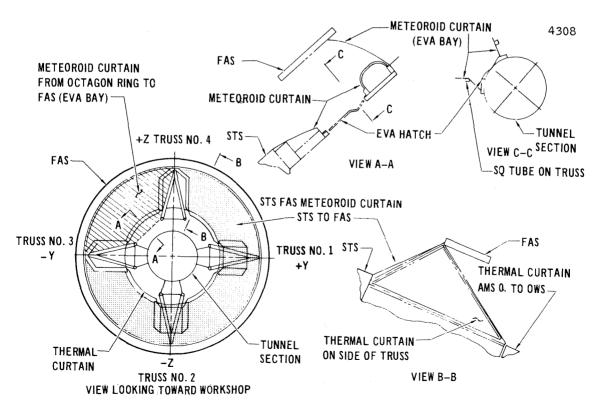
Figure 2.4.4-31 AM Thermal Installation
