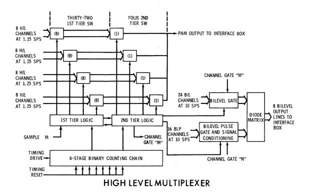
Figure 2.6.4-11 Multiplexer Block Diagram
