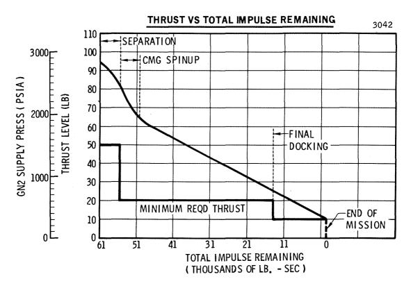
Figure 2.3.6-1 Thruster Versus Impulse Remaining
