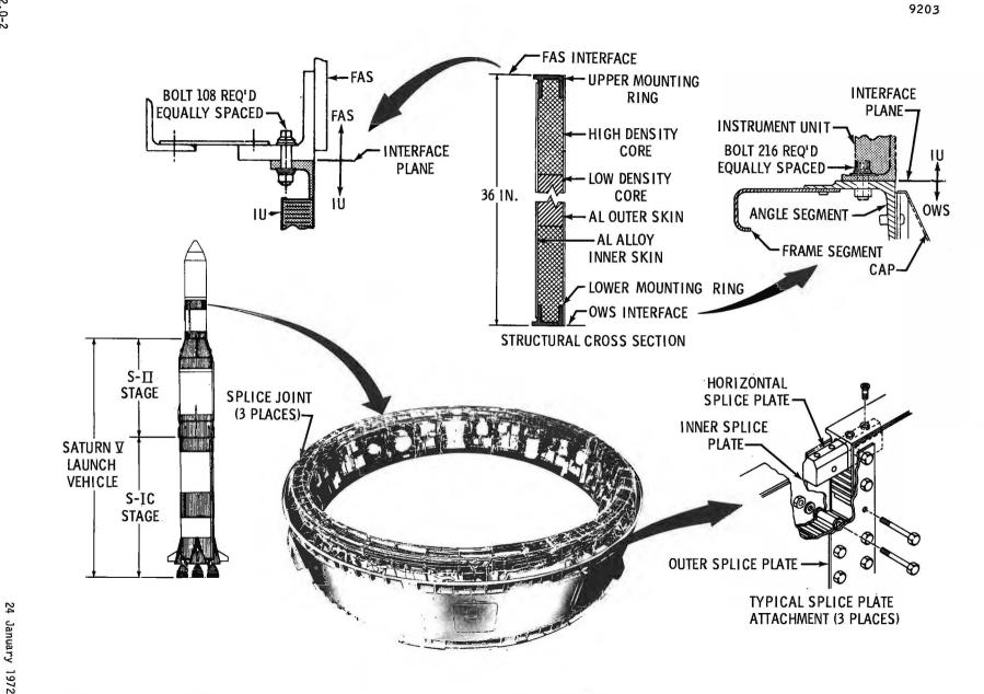
Figure 2.0.2-1 Instrumentation Structural Arrangement
