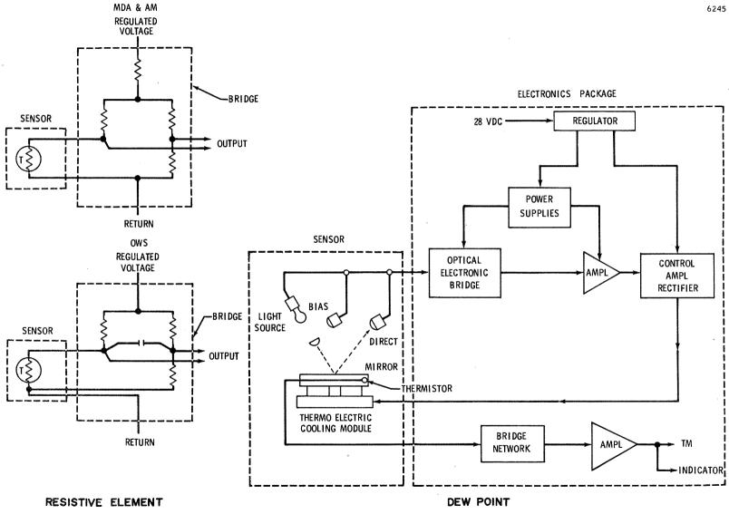
Figure 2.6.4-5 Temperature Transducers
