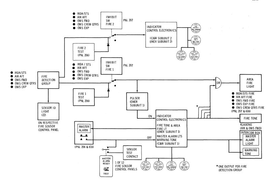
Figure 2.8.3-7 Fire Detection Functional
