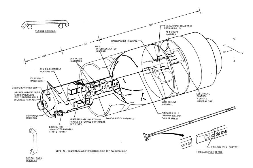
Figure 2.5.3-3 Fixed Crewman Hand Restraints - Internal
