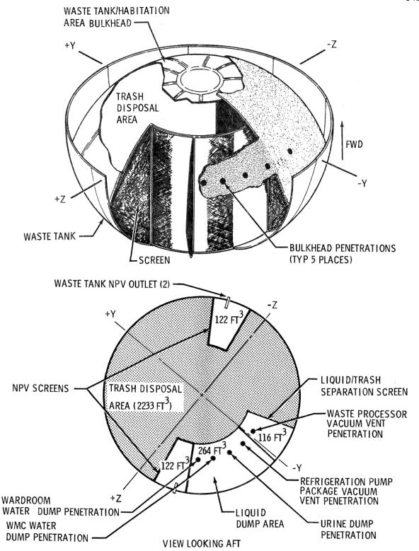
Figure 2.5.14-4 Waste Tank Liquid Dump Area
