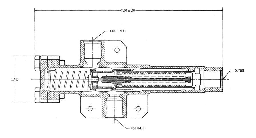
Figure 2.4.4-43 Temperature Control Valve -- 47°F
