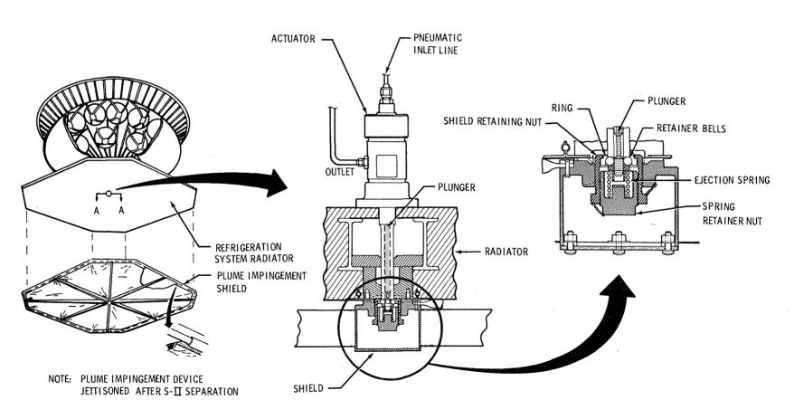
Figure 2.0.10-21 Radiator Plume Impingement Shield
