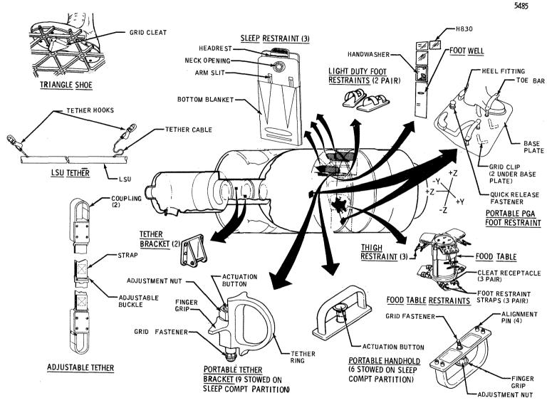
Figure 2.5.3-2 Crewman Restraints - Internal
