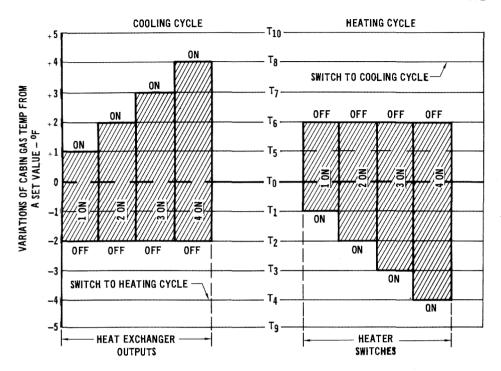
Figure 2.4.4-38 Automatic Temperature Control Logic
