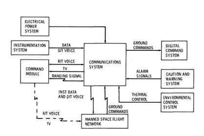
Figure 2.2.2-1 Communication System Interfaces
