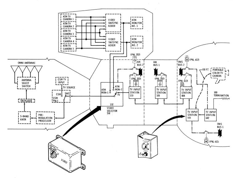
Figure 2.2.3-3 Television Subsystem Configuration
