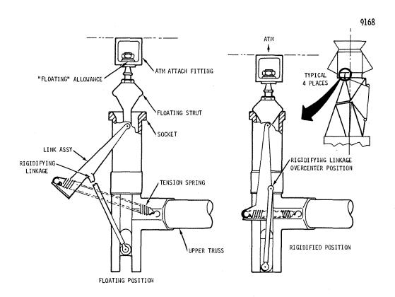
Figure 2.0.6-3 Rigidifying Mechanism
