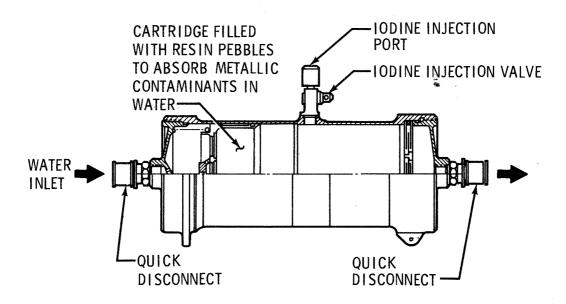
Figure 2.5.12-10 Cat Ion Cartridge
