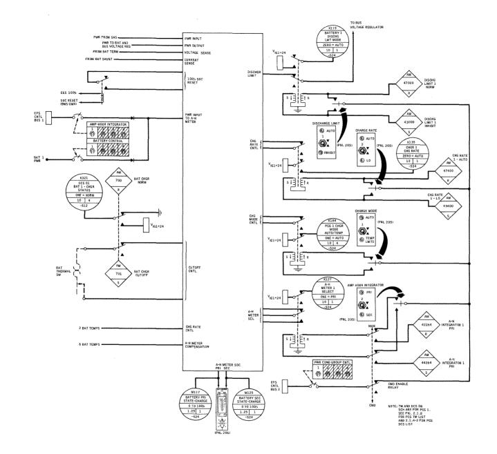
Figure 2.1.3-9 Simplified Battery Charger Diagram
