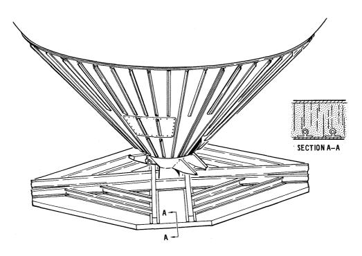
Figure 2.4.4-81 Refrigeration System Radiator
