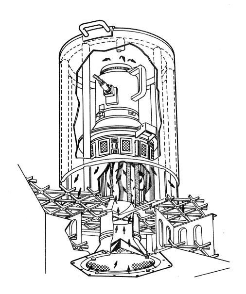
Figure 2.4.4-56 WMC Fan Assembly
