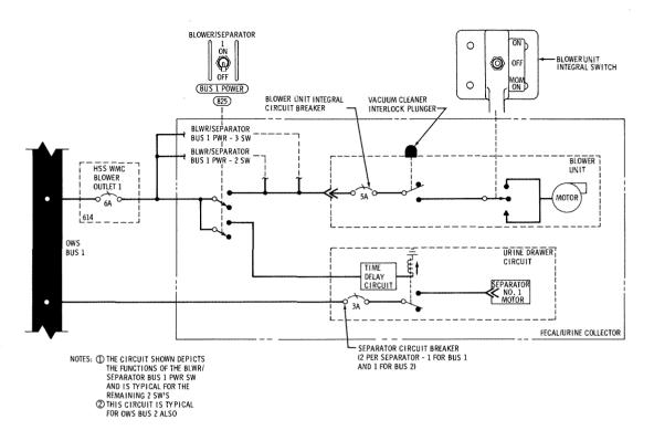
Figure 2.5.11-9 Fecal/Urine Collector -- Schematic
