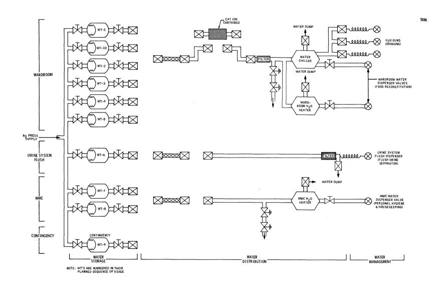
Figure 2.5.12-1 Water System -- Functional Flow
