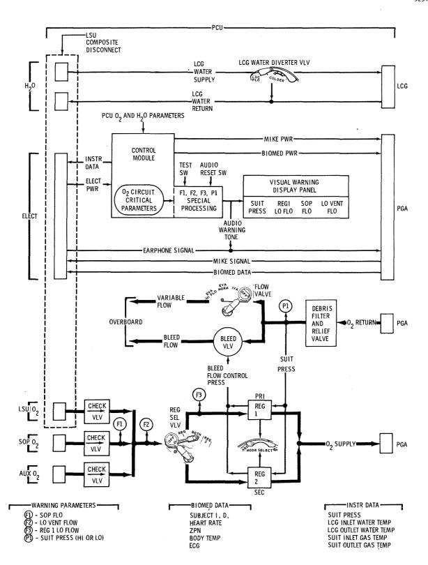
Figure 2.5.7-9 ALSA PCU -- Functional Diagram
