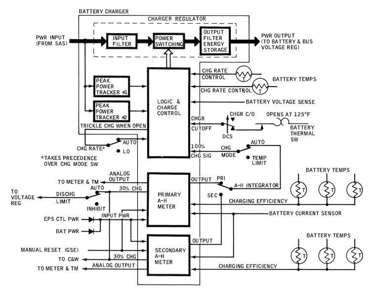
Figure 2.1.4-9 Battery Charger Functional Diagram
