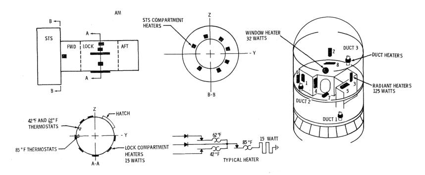
Figure 2.4.4-28 Electrical Heater Locations
