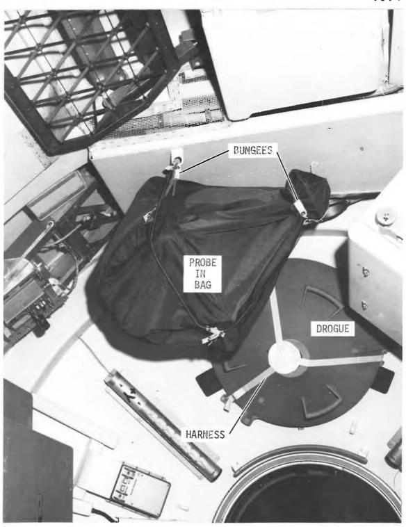
Figure 2.9-5 Drogue and Probe Stowage
