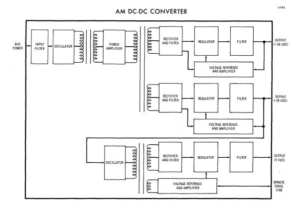
Figure 2.6.4-2 AM DC-DC Converter
