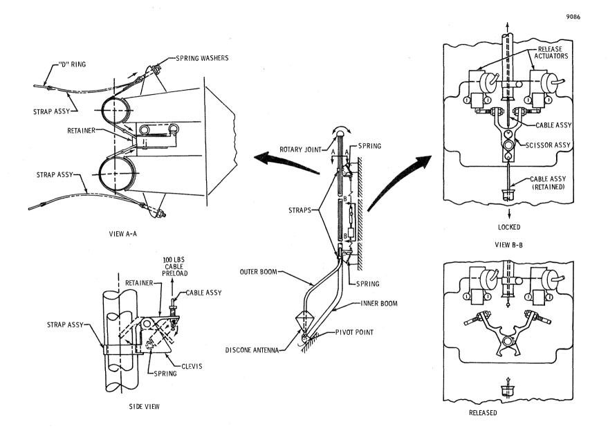
Figure 2.0.4-3 Discone Antenna Release Mechanisms
