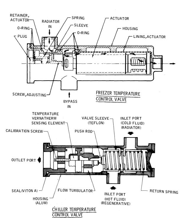
Figure 2.4.4-83 Temperature Control Valves
