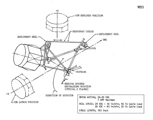
Figure 2.0.6-8 DA Rotation Mechanism
