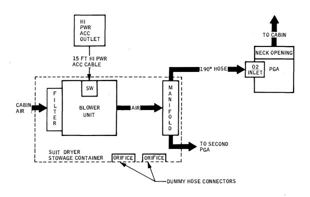
Figure 2.5.7-12 Suit Dryer -- Functional Diagram
