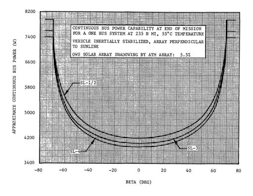
Figure 2.1.4-5 AM-OWS Electrical Power Capability
