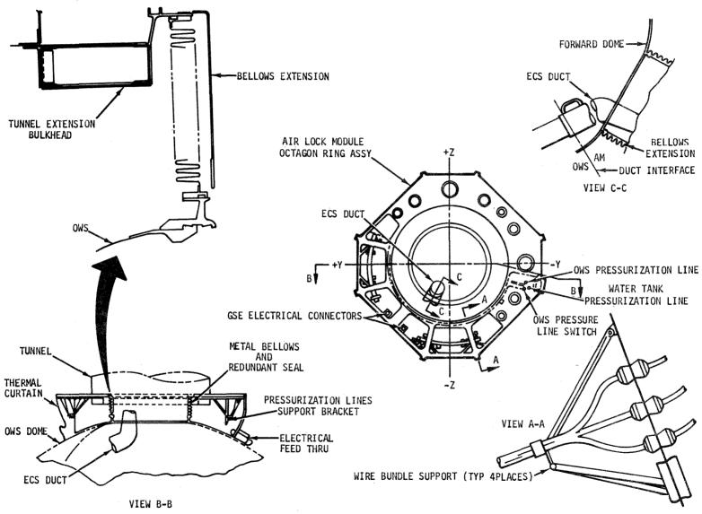
Figure 2.0.8-13 Flexible Tunnel Extension Assembly
