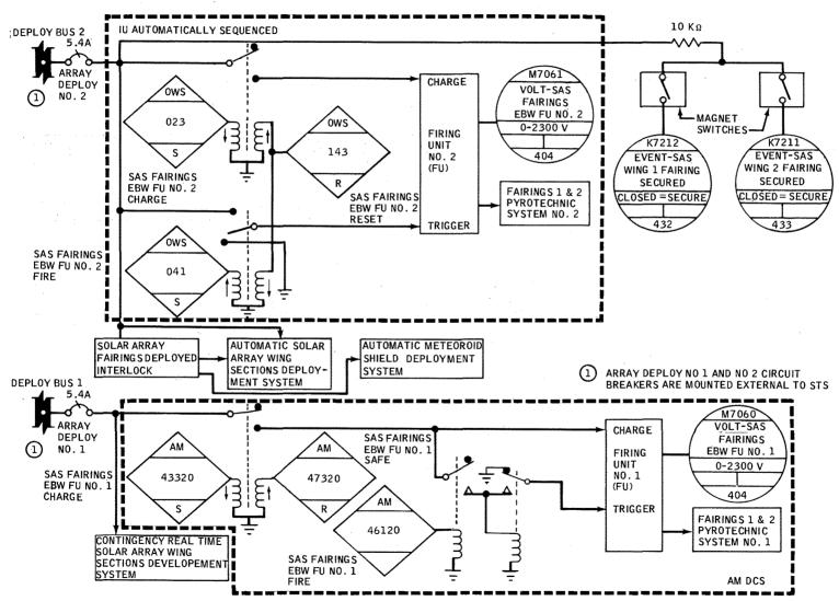
Figure 2.0.10-27 Solar Array Fairings 1 and 2 Deployment Systems
