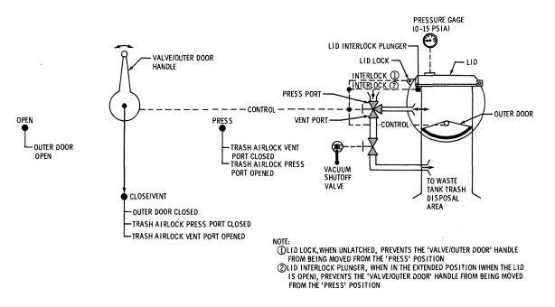
Figure 2.5.9-3 Trash Disposal Airlock -- Functional Diagram
