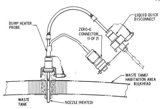
Figure 2.5.14-2 Dump Heater Probe
