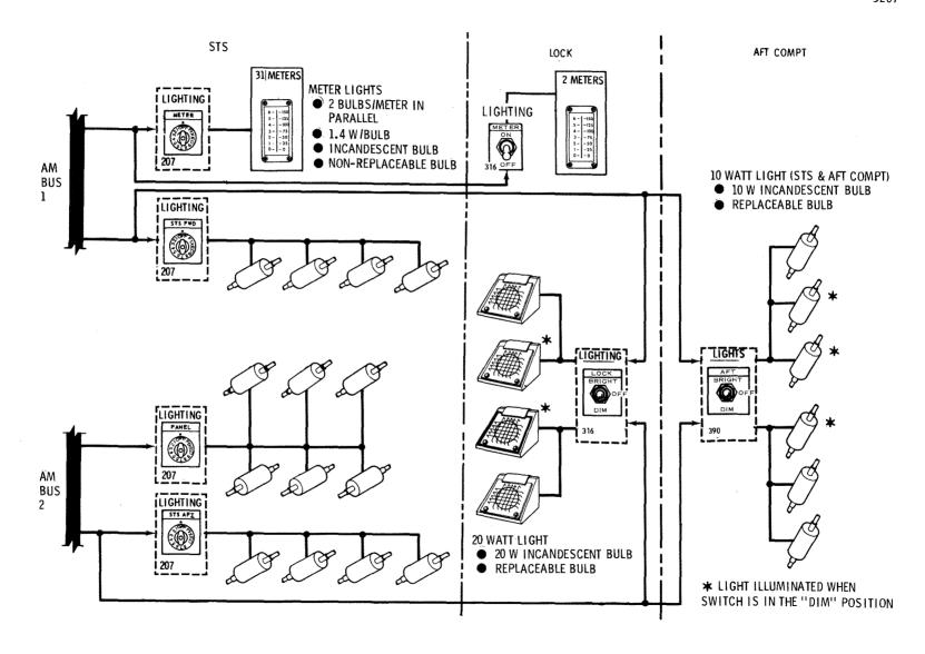
Figure 2.5.4-12 AM Internal Lighting -- Functional Diagram
