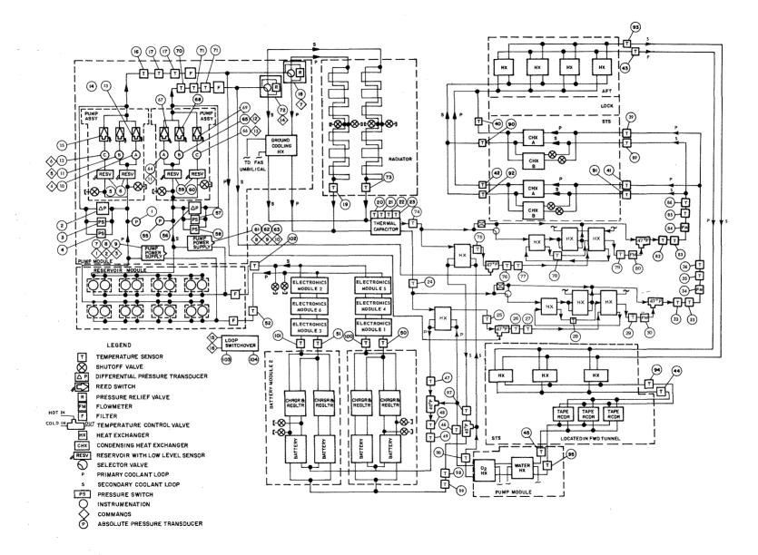
Figure 2.4.4-21 Coolant System
