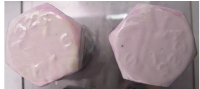
Nut and bolt set up for crevice corrosion testing. The pictures show results after 600 hour of salt fog exposure 70
