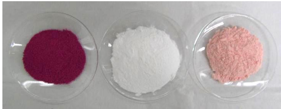
Free flowing powder samples of hydrophobic-core microcapsules. The core contents of these microcapsules are Rhodamine B (on the left), Phenolphthalein (in the middle), and a universal pH indicator (on the right).
