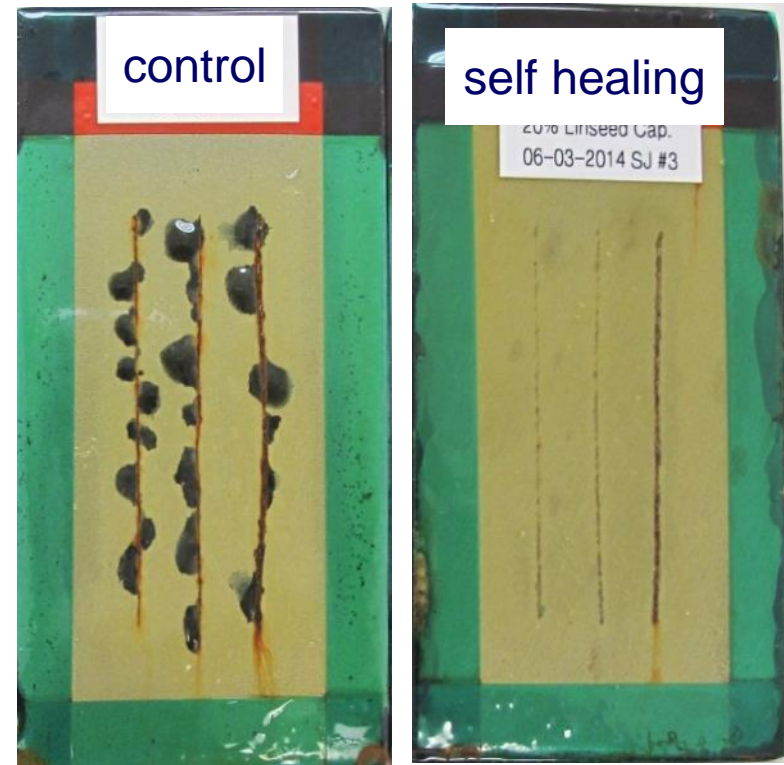
Control and self healing paint coated steel panels after 1000 hours of salt fog testing.
