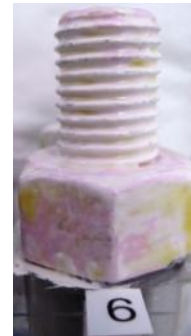
Nut and bolt set up for crevice corrosion testing. The pictures show results after 600 hour of salt fog exposure 70
