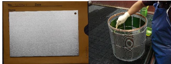
Fig. 4: a) Demonstration fatigue crack specimen and b) demonstration configuration.
