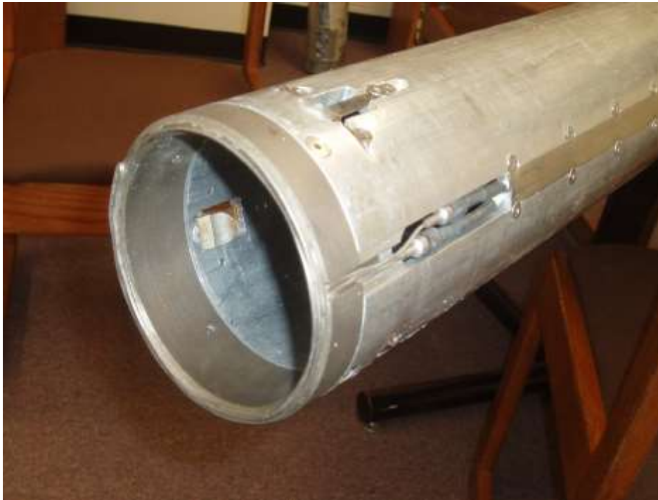
A thermal drill head showing the absence of cutters. Thermal drills use a heating element to melt an annulus around the ice to be cored. —Credit: Tony Wendricks, Univ. Wisconsin
