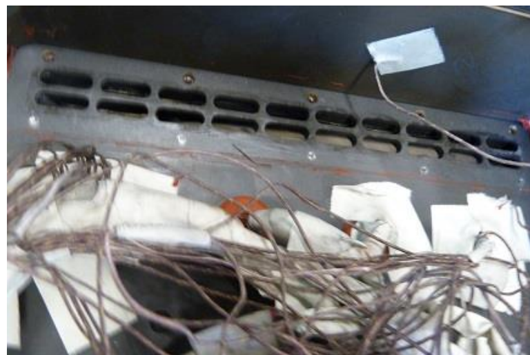
Minor collateral damage observed, particulates and flame remained internal to battery enclosure
