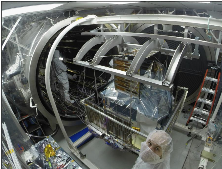
Figure 1 8x15 TVAC Chamber Test Facility
